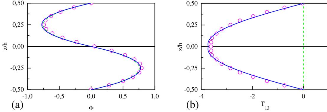
Fig.3 : Force density applied on the top face of a piezoelectric bimorph in closed circuit for  $L/h = 10$ . Plate model (full line), finite element (small circles) and simplified plate model (dashed-line).
