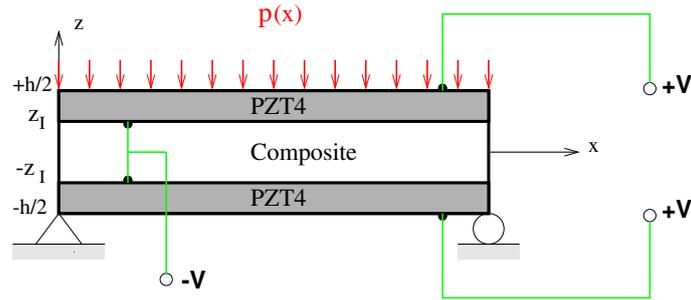
Fig.8 : Piezoelectric sandwich plate with intermediate electrodes.
