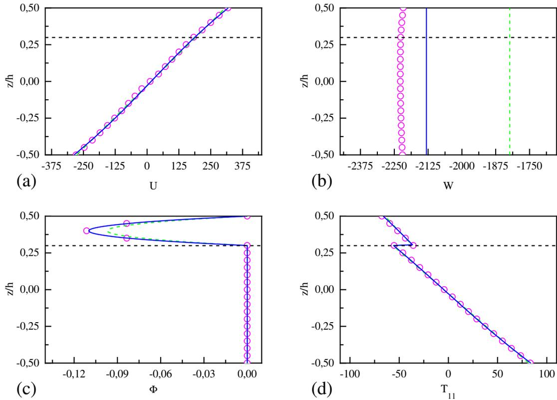
Fig.6 : Force density applied on the top face of a piezoelectric bi-layer in closed circuit for  $L/h = 10$ .
