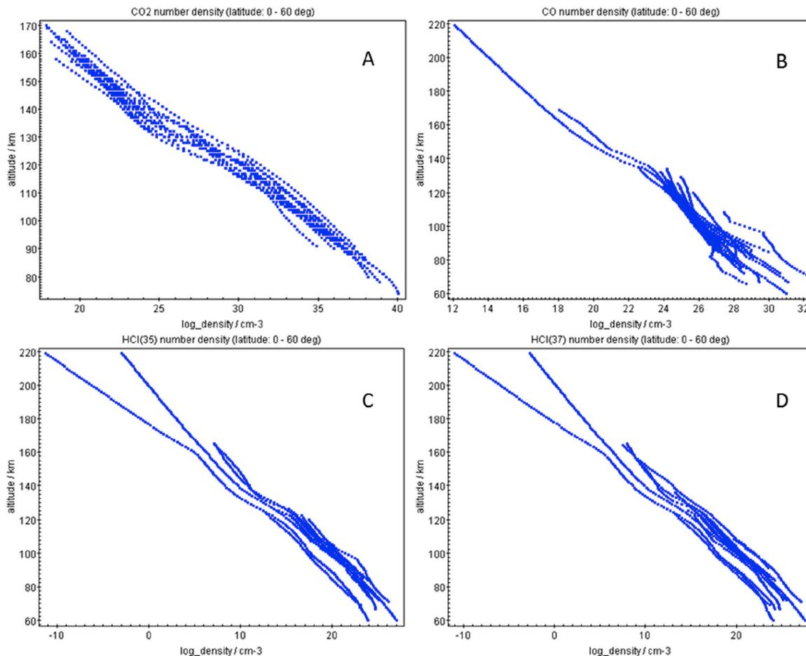
Fig. 4. Number density profiles for CO<sub>2</sub> (panel A), CO (panel B), H<sup>35</sup>Cl (panel C) and H<sup>37</sup>Cl (panel D) located between 0 and 60° of latitude (Northern hemisphere). For each species, the corresponding plot contains all vertical profiles retrieved and accessible through the *soir* database.
