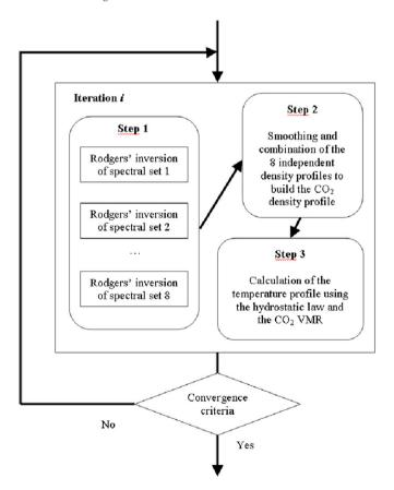
Fig. 2. Working principle of the ASIMAT program to derive profiles from the spectra of SOIR.
