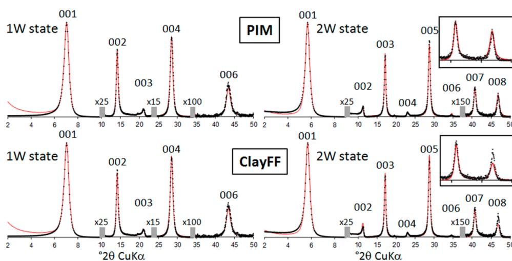
**Figure 4.** Experimental (black crosses) and calculated (red lines) intensities of 00l reflections for hectorite under monohydrated (1W-left) and bihydrated (2W-right) state and using PIM (top) or ClayFF (bottom) models. The vertical gray bars indicate a modified scale factor for the high-angle regions as compared to the low-angle part of the patterns. 00l reflections are indexed on the top part of the figure. For 2W state, a zoom of the 007 and 008 reflections is shown for both models.
