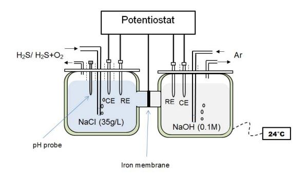
Figure 2: Experimental set up (Devanathan-Stachurski type cell).
