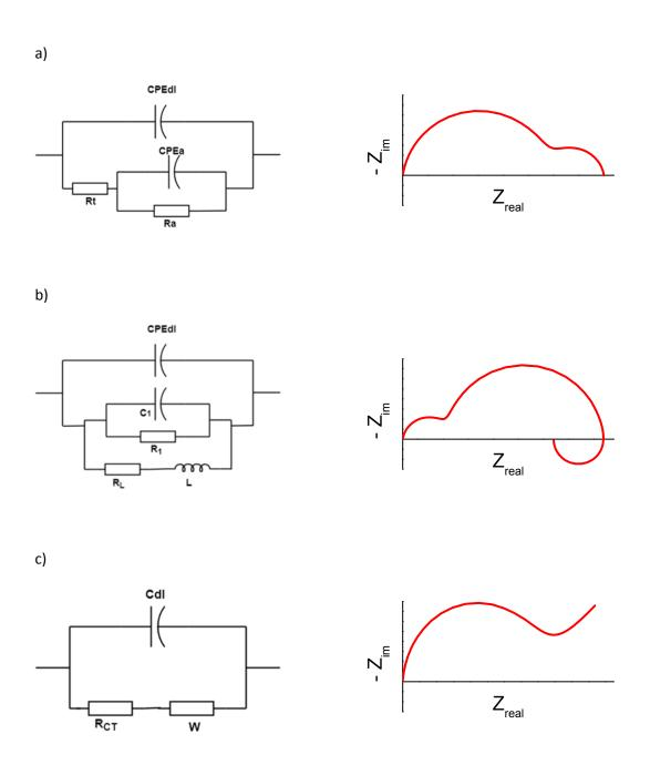
Figure 1: Equivalent circuits and corresponding impedance diagram used in the literature to describe iron corrosion in presence of  $H_2S$  [8,9,13]. For the sake of simplicity, electrolyte resistance was removed from these equivalent circuits.
