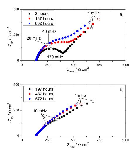
Figure 4: Nyquist diagrams of pure iron exposed to a 35 g/L NaCl solution saturated with 1 bar H<sub>2</sub>S at 24 °C for short (a) and long (b) exposure times.
