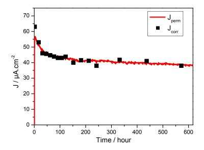
Figure 11: Comparison of  $J_{perm}$  with  $J_{corr}$  determined from  $R_t$  values determined by EIS fitting with the model of **Erreur! Source du renvoi introuvable.**
