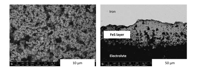
Figure 6: SEM observation of corrosion deposits formed at iron surface after 620 hours exposure to a 35 g/L NaCl solution saturated with 1 bar  $H_2S$  at 24  $^\circ$  C.
