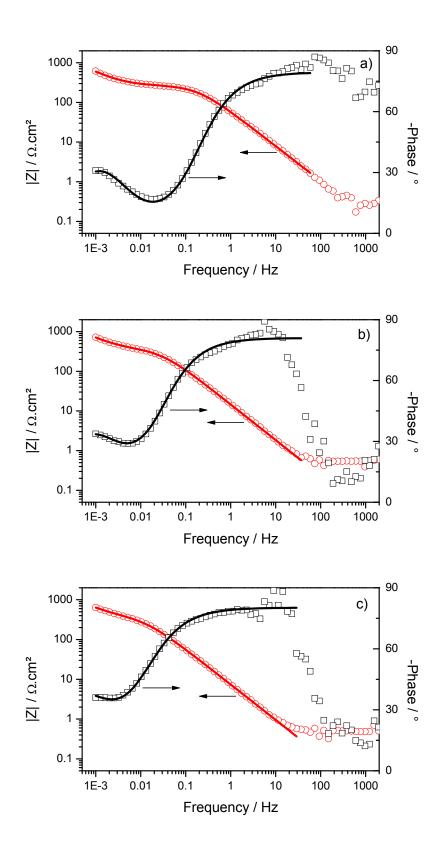
Figure 8: Comparisons between experimental (open symbols) and fitted impedance (lines) measured after 2 hours (a), 47 hours (b) and 152 hours (c) exposure, using the equivalent circuit of Figure 1.a.
