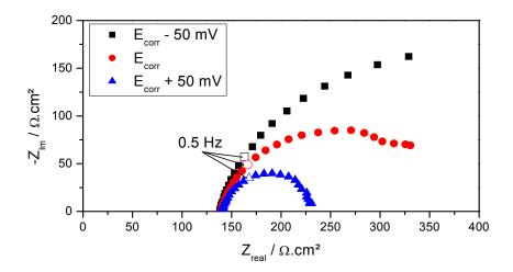
Figure 5: Nyquist diagram of pure iron exposed to a 35 g/L NaCl solution saturated with 1 bar H<sub>2</sub>S at 24 °C. Measurements at  $E_{corr}$  – 50 mV,  $E_{corr}$ , and  $E_{corr}$  + 50 mV.
