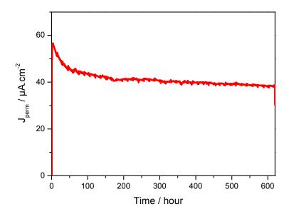
Figure 7: Hydrogen permeation for a 0.5 mm thick pure iron membrane exposed to a 35 g/L NaCl solution saturated with 1 bar  $H_2S$  at 24  $^{\circ}C$ .
