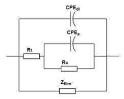
Figure 9: Equivalent circuit for the corrosion of pure iron in  $H_2S$  containing environment with the formation of a conductive and porous FeS layer.
