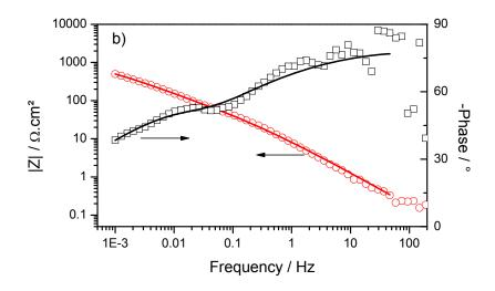
Figure 10: Comparisons between experimental (open symbols) and fitted impedance (lines) measured after 437 hours (a) and 572 hours (b) exposure, using the equivalent circuit of **Erreur! Source du renvoi introuvable.**.
