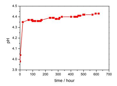
Figure 3: pH evolution of test solution consisting of 35 g/L NaCl solution saturated with 1 bar  $H_2S$  at 24 °C, with iron coupons exposed to corrosion.
