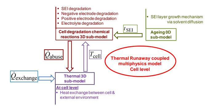
Fig. 1. Thermal runaway coupled multiphysics model.
