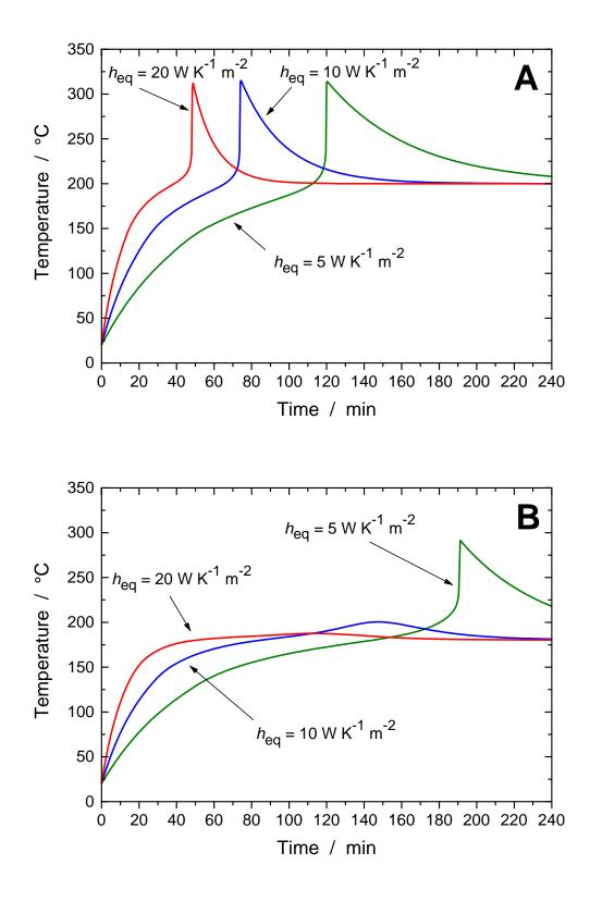
**Fig. 7.** Influence of the equivalent heat transfer coefficient on the average surface temperature of a fresh A123 cell:  $T_{\text{ext}} = 200^{\circ}\text{C}$  (A),  $T_{\text{ext}} = 180^{\circ}\text{C}$  (B).
