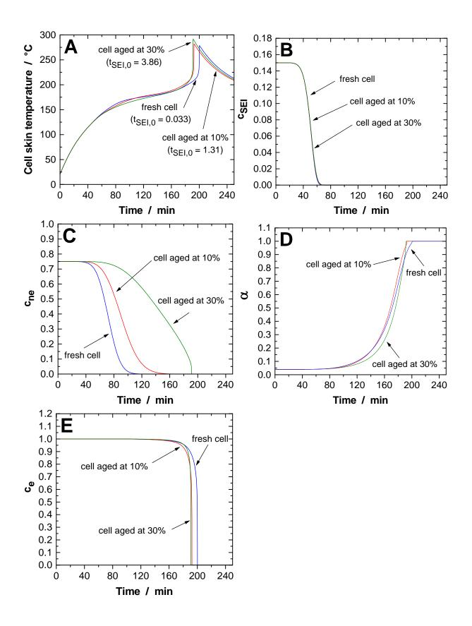
**Fig. 8.** Simulated evolution of the cell average surface temperature (A) and dimensionless concentrations of the reactive species (B to E) during the oven test ( $T_{\text{ext}} = 180^{\circ}\text{C}$ ,  $h_{\text{eq}} = 5 \text{ W K}^{-1} \text{ m}^{-2}$ ).
