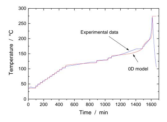
**Fig. 3.** Comparison of the simulated average surface temperature of a fresh A123 battery cell with the experimental data in Fig. 2.
