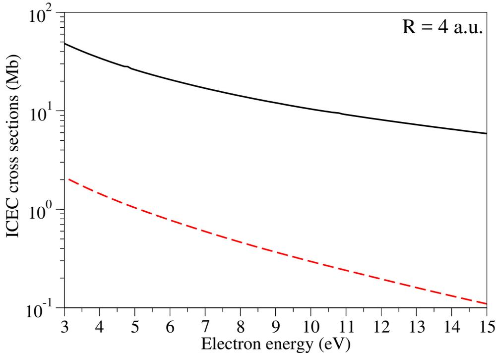
FIG. 1. Absolute ICEC cross sections (in Mb) as functions of the electron energy for  $\text{Ne}^+\text{-He}$  at the interatomic distance  $R = 4$  a.u. This value is about the equilibrium interatomic distance of  $\text{Ne}^+\text{-He}$ . The full black line represents results from the R-Matrix calculations and the red dashed line the cross sections given by the asymptotic formula (see text).
