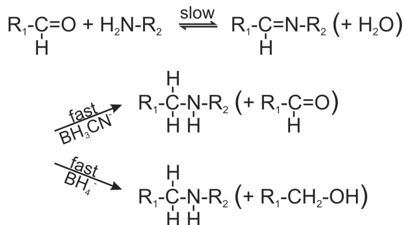
Fig. (8). Reaction scheme of the Schiff base formation and its in situ reduction with sodium borohydride (NaBH 4 ) or sodium cyanoborohydride (NaBH 3 CN). With both reducing agents, the overall crosslinking reaction is rate-limited by the formation of the iminium moiety, not by its in situ reduction.
