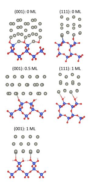
**Fig. 4** Zinc deposits on dry (0 ML), partially (0.5 ML) and fully (1 ML) hydroxylated (001) (left) and (111) (right) surfaces of the  $\beta$ -cristobalite. The density d of interface silanols increases from top to bottom, with  $d_{\rm OH}^{001}(0.5 {\rm ML}) \sim d_{\rm OH}^{111}(1 {\rm ML})$ . Si, Zn, O, and H atoms are represented by large blue and grey, medium red, and small white balls, respectively.
