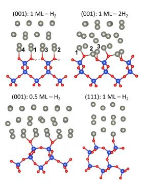
**Fig. 6** Relaxed structure of the partially and fully dehydrogenated zinc/silica interfaces. Top: fully hydroxylated (001) interfaces after desorption of one (left) and two (right) hydrogen molecules. Bottom: partially hydroxylated (001) (left) and fully hydroxylated (111) (right) interfaces after desorption of one hydrogen molecule. Si, Zn, O, and H atoms are represented by large blue and grey, medium red, and small white balls, respectively.
