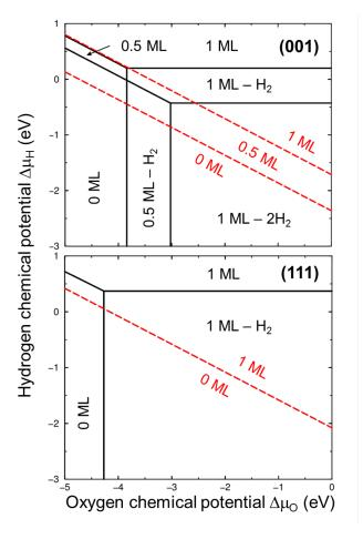
**Fig. 7** Stable zinc/ $\beta$ -cristobalite (001) and (111) interface configurations, as a function of oxygen and hydrogen chemical potentials  $\Delta\mu_O$  and  $\Delta\mu_H$  (eV). As a reference, red labels and red dashed lines recall the corresponding configurations in the absence of zinc.
