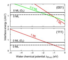
**Fig. 5** Interface energies ( $J/m^2$ ) of dry and hydroxylated zinc/β-cristobalite interfaces, as a function of water chemical potential  $Δμ_{H_2O}$  (eV). Results for the (001) and (111) interfaces are given in the top and bottom panels, respectively.
