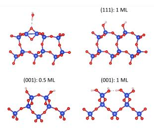
**Fig. 2** Fully and partially hydroxylated surfaces of β-cristobalite. Top: molecularly (left) and dissociatively (right) adsorbed 1 ML of water on the (111) surface. Bottom: dissociative adsorption of 0.5 ML (left) and 1 ML (right) of water on the (001) surface. Si, O, and H atoms are represented by large blue, medium red, and small white balls, respectively.
