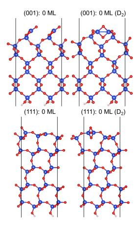
Fig. 1 Relaxed bare stoichimetric (001) (top) and (111) (bottom) surfaces of  $\beta$ -cristobalite: configurations with broken (left panels) and intact (right panels) surface two-member siloxane rings (D<sub>2</sub>). Si, O, and H atoms are represented by large blue, medium red, and small white balls, respectively and surface unit cells used in the calculations are indicated.
