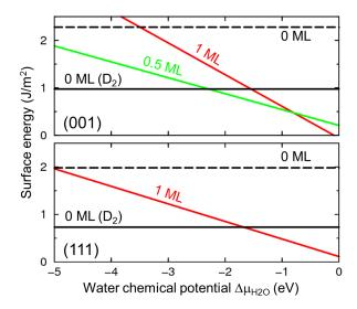
**Fig. 3** Surface energies (J/m²) of hydroxylated surfaces of  $\beta$ -cristobalite, as a function of water chemical potential  $\Delta \mu_{H_2O}$  (eV). Results for (001) and (111) terminations are given in top and bottom panels, respectively. The surface energies of bare surfaces (0 ML) with both intact (D₂) and broken (dashed line) surface siloxane rings are recalled.
