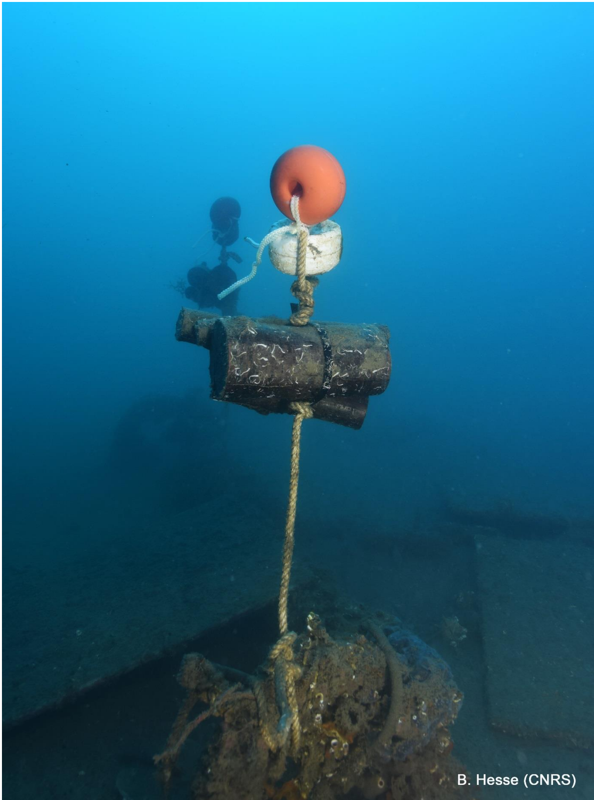
Figure S1: Experimental setup. Image of the alder wood packs at the study site within the Bay of Banyuls-sur-Mer, Mediterranean Sea, France.
