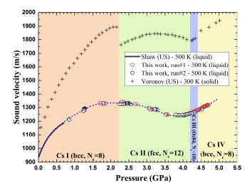
FIG. 1. (color online) Longitudinal wave velocities of l-Cs as a function of pressure for the present work (T=500K, two runs, black and red open circles; dotted line, as guides for the eyes), plotted along with low-pressure ultrasonic data on l-Cs at 500 K from Ref<sup>28</sup> (black line) and ultrasonic measurements on solid-Cs at 300 K from Ref<sup>29</sup> (crosses). The maximal uncertainties associated with the relative sound velocity  $\Delta v_l/v_l$  is less than  $0.5\%^{22,26}$ .
