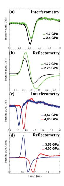
FIG. 2. (color online) Reflectivity change of l-Cs at 500 K as a function of the optical probe-pulse time delay. The modification of the optical reflectivity due to the acoustic strain has been recorded around 2 GPa using two types of detection, reflectometry (a) and interferometry (b). Same but around 4 GPa are given in (c) and (d) respectively. The pulse shape qualitatively varies (shifted in phase by about  $\pi$ ) only in the vicinity of 4 GPa and using a reflectometric detection.
