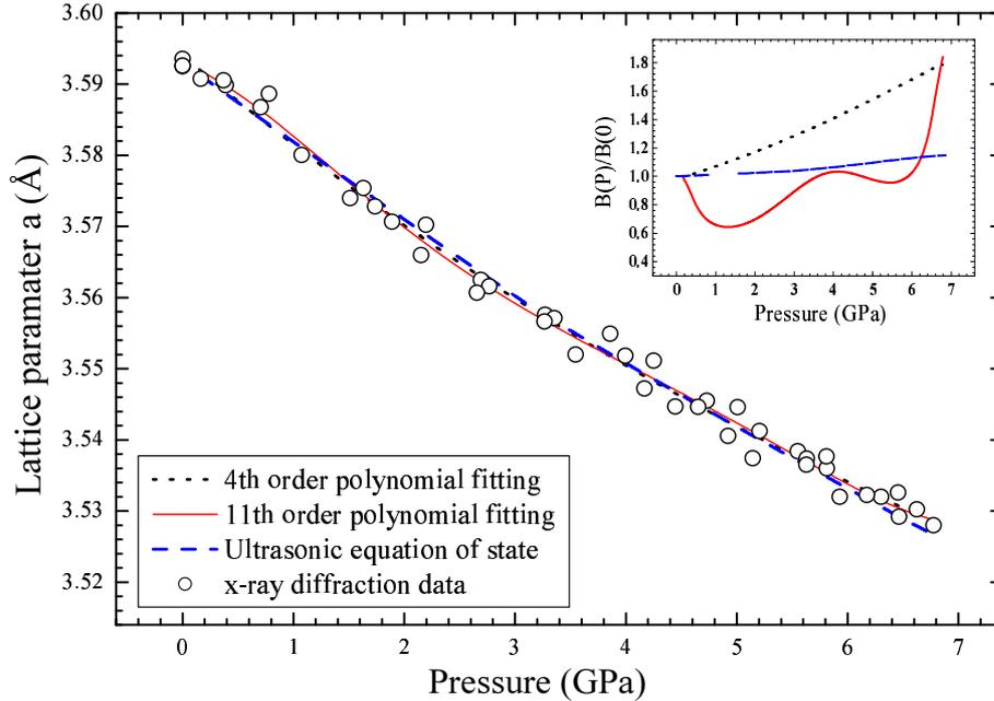
FIG. 3: Pressure dependence of polycrystalline  $\text{Fe}_{64}\text{Ni}_{36}$  lattice parameter (circles) with 11th and 4th order polynomial fittings (solid and dot lines respectively). Dashed line : equation of state using the ultrasonic  $B'(P)$  data and  $3.5935(8)$  Å. Inset : comparison between ultrasonic results and bulk modulus derived from the polynomial fitting curves using the thermodynamical definition of  $B$ .
