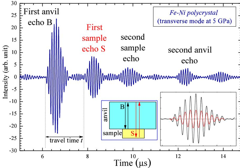
FIG. 1: Ultrasonic spectrum of  $\text{Fe}_{64}\text{Ni}_{36}$  at 5 GPa. The first echo is the first reflection at the anvil/sample interface (B) and the second echo (S) the first reflection from the far end of the sample. The classical pulse echo superposition method (inset) using a signal cross correlation section between the B and S echoes is used to determine the travel time  $t$ .
