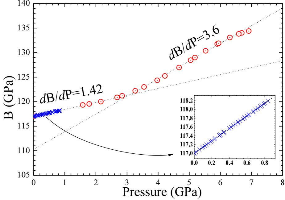
FIG. 2: Pressure dependence of bulk moduli in poly-crystalline  $\text{Fe}_{64}\text{Ni}_{36}$ . Between 0 and 1.0 GPa, experiments using the piston-cylinder apparatus (cross) supplement the high pressure Paris-Edinburgh measurements (open circles). The uncertainties in pressure and bulk modulus are within the symbol size.
