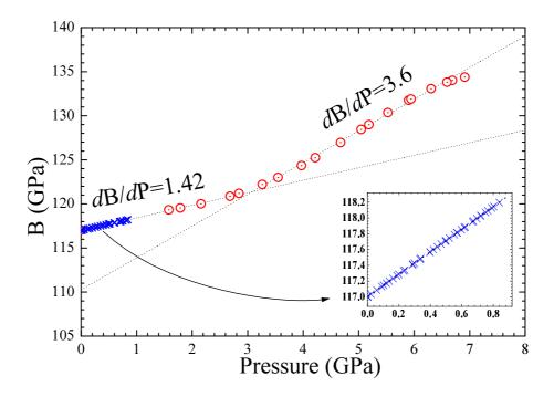
FIG. 2: Pressure dependence of bulk moduli in poly-crystalline Fe<sub>64</sub>Ni<sub>36</sub>. Between 0 and 1.0 GPa, experiments using the piston-cylinder apparatus (cross) supplement the high pressure Paris-Edinburgh measurements (open circles). The uncertainties in pressure and bulk modulus are within the symbol size.
