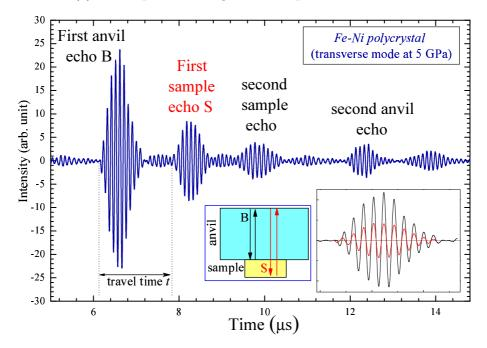
FIG. 1: Ultrasonic spectrum of  $Fe_{64}Ni_{36}$  at 5 GPa. The first echo is the first reflection at the anvil/sample interface (B) and the second echo (S) the first reflection from the far end of the sample. The classical pulse echo superposition method (inset) using a signal cross correlation section between the B and S echoes is used to determine the travel time t.
