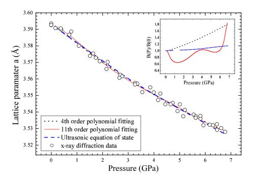
FIG. 3: Pressure dependence of polycrystalline  $Fe_{64}Ni_{36}$  lattice parameter (circles) with 11th and 4th order polynomial fittings (solid and dot lines respectively). Dashed line: equation of state using the ultrasonic B'(P) data and 3.5935(8)  $\mathring{A}$ . Inset: comparison between ultrasonic results and bulk modulus derived from the polynomial fitting curves using the thermodynamical definition of B.
