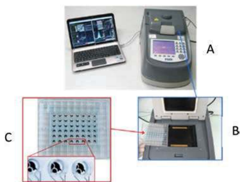
Scheme 1 (A) Overview of the real-time electrochemical qPCR prototype that monitors, in parallel, up to 48 PCR reactions. (B) Flat Peltier-heating block and its two 72-pin connectors mounted in a standard PCR thermocycler. (C) Disposable 48-well electrochemical microplate (the inset shows a zoom on the electrochemical microwells equipped at their flat bottom with three screen-printed electrodes).
