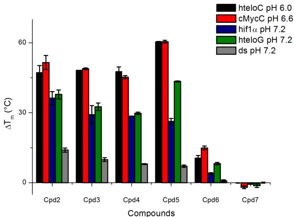
**Figure 8:** Stabilization of different DNA structures (0.2  $\mu$ M) in 10 mM sodium cacodylate, 100 mM NaCl when dosed with 50  $\mu$ M concentrations of dithiocarbamate complexes **2** - **7**. Data represents the average and standard deviations of two experiments.
