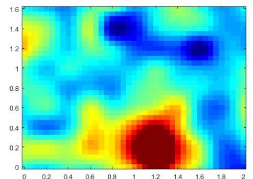
Correlation coefficient of a footfall on a concrete slab ( $2 \times 1.6m^2$ )
