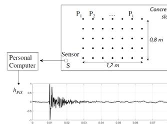
Concrete slab discretization
