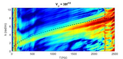
Feat of the dispersion curve of the concrete slab of the laboratory (only  $A_0$  mode is visible)
