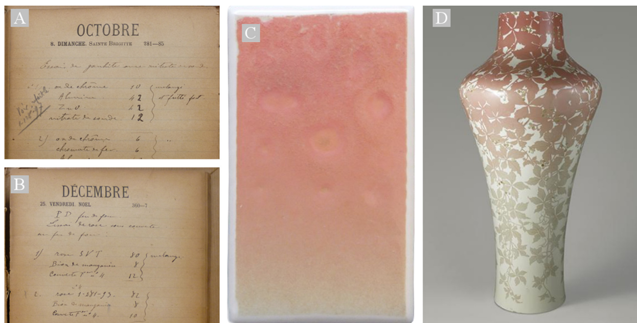
Fig. 1. From laboratory tests to the production of objects. (A–B) Extract from the laboratory notebooks of the years 1893 and 1896, referring to the synthesis of a gahnite with chromium type pigment on October 8th, and its test in a porcelain decoration on December 25th, respectively. (C) Porcelain slab composed of the porcelain decoration prepared on December 25th, 1896. The reference of the sample appears on the back of the slab (not shown). (D) Vase de Chagny A (1899) from the collection of the “Cité de la céramique”, MNC12652, dimensions: 120 cm (height), 55 cm (diameter). ©RMN-Grand Palais.
