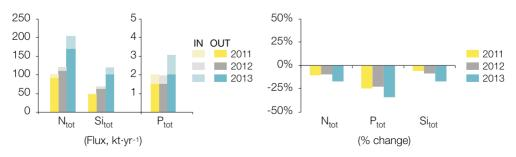
**Fig. 5.** The estuarine filter, from Poses to Le Havre, for three different years: 2011 (dry), 2012 (average), and 2013 (wet). The absolute nutrient fluxes entering and leaving the estuary are shown on the left, and the percentage of change is shown on the right. N<sub>tot</sub> refers to nitrogen, P<sub>tot</sub> to phosphorus, and Si<sub>tot</sub> to silica. [Color figure can be viewed at wileyonlinelibrary.com]
