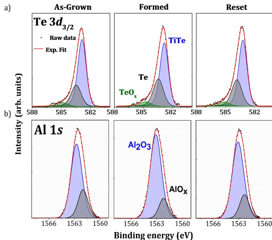
**Figure 3.** (a) Te  $3d_{3/2}$  and (b) Al  $1s$  core level peaks obtained by HAXPES at 6.9 keV on as-grown, formed and the reset sample of the TaN/TiTe/ $\text{Al}_2\text{O}_3$ /Ta stack.
