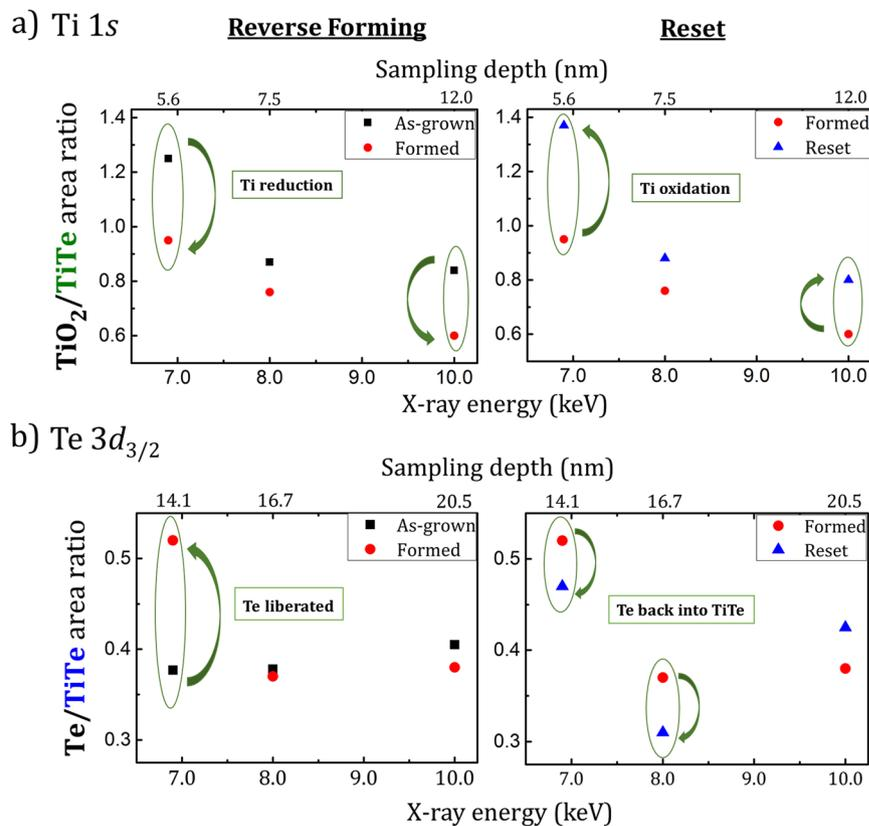
**Figure 4.** (a)  $\text{TiO}_2/\text{TiTe}$  area ratios extracted from the Ti 1s line and (b) Te/TiTe area ratios extracted from Te  $3d_{3/2}$  measured at 6.9, 8 and 10 keV for as-grown formed and reset samples.
