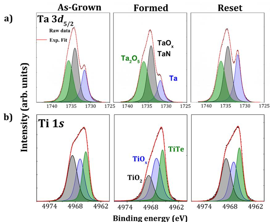
**Figure 2.** (a) Ta  $3d_{5/2}$  and (b) Ti  $1s$  core level peaks obtained by HAXPES at 6.9 keV on as-grown, formed and reset sample of the TaN/TiTe/Al<sub>2</sub>O<sub>3</sub>/Ta stack.
