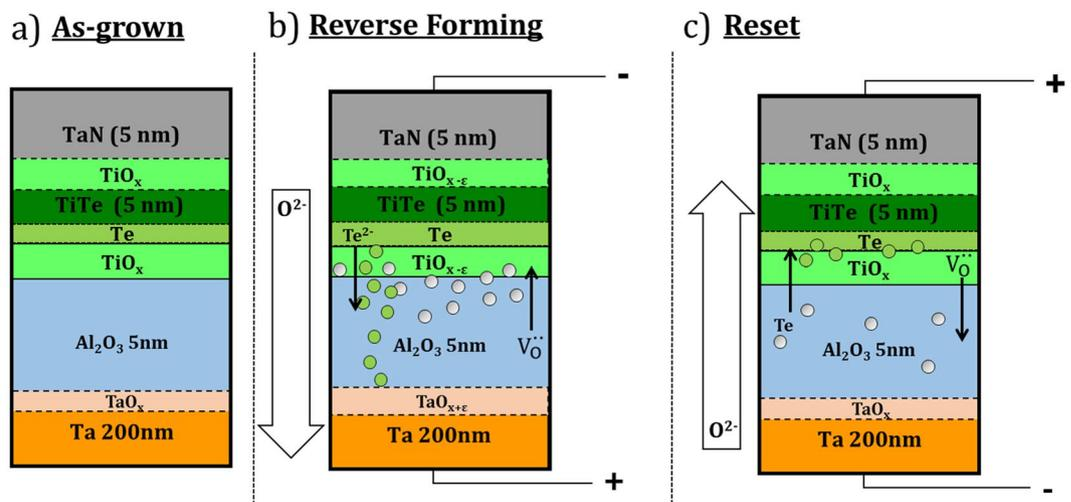
**Figure 6.** Schematic of the (a) as-grown sample and the redox processes and matter transport taking place during (b) forming and (c) reset in the TaN/TiTe/Al<sub>2</sub>O<sub>3</sub>/Ta stack.
