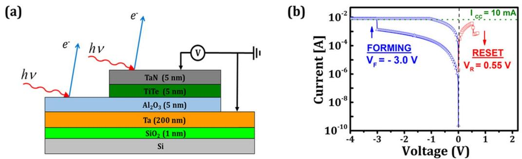
**Figure 1.** (a) Schematic of the TaN/TiTe/Al<sub>2</sub>O<sub>3</sub>/Ta device structure of the HAXPES measurements and schematic of the setup for electrical characterization (b) I-V curve for the forming and the reset of the TaN/TiTe/Al<sub>2</sub>O<sub>3</sub>/Ta stack.
