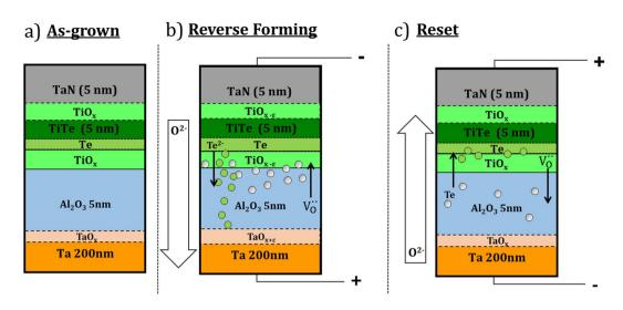
Figure 6. Schematic of the (a) as-grown sample and the redox processes and matter transport taking place during (b) forming and (c) reset in the TaN/TiTe/Al<sub>2</sub>O<sub>3</sub>/Ta stack.
