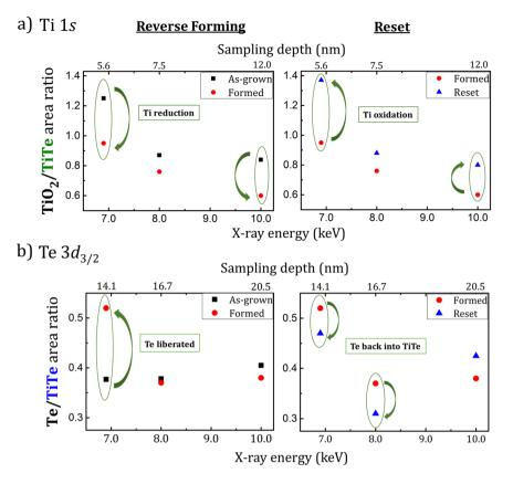
**Figure 4.** (a)  $TiO_2/TiTe$  area ratios extracted from the Ti 1*s* line and (b) Te/TiTe area ratios extracted from Te  $3d_{3/2}$  measured at 6.9, 8 and 10 keV for as-grown formed and reset samples.
