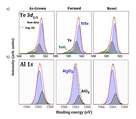
**Figure 3.** (a) Te  $3d_{3/2}$  and (b) Al 1s core level peaks obtained by HAXPES at 6.9 keV on as-grown, formed and the reset sample of the TaN/TiTe/Al<sub>2</sub>O<sub>3</sub>/Ta stack.
