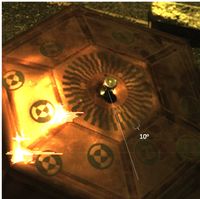
Figure 11: Picture of the gnomon and target above the SEIS seismometer.
