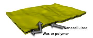
**Figure 20**: Schematic representation of the sandwiched thin film structures in which a nanocellulose film, which offers high resistance to oxygen permeation when dry, is sandwiched between a pair of water-resistent layers.
