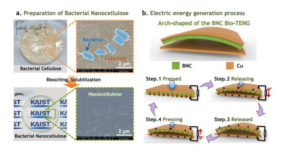
**Figure 23.** (a) BNC is regenerated and solubilized to form a flexible and transparent film. (b) Energy is generated using mechanical force. A copper foil is used as a current collector and a source of friction with the BNC layer. Reproduced with permission from ref. 436, Copyright 2017, Elsevier.
