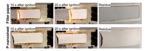
**Figure 25**: Snapshots of filter paper (top) and P-nanosheet (bottom) taken at fixed times during the flammability test. (Reprinted with permission from ref. 136, Copyright 2015, American Chemical Society).
