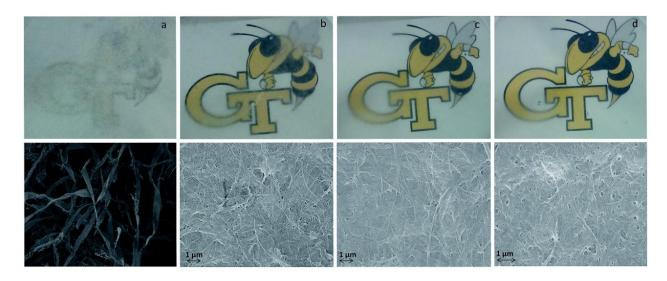
**Figure 7:** Photos of cellulose films showing their increasing transparency and corresponding SEM images of (a) disintegrated cellulose, (b) PFI cellulose refining, and (c) 20 passes or (d) 60 passes of micro-grinding in the super mass collider. Reproduced with permission from ref. 98, Copyright 2015, Royal Society of Chemistry.
