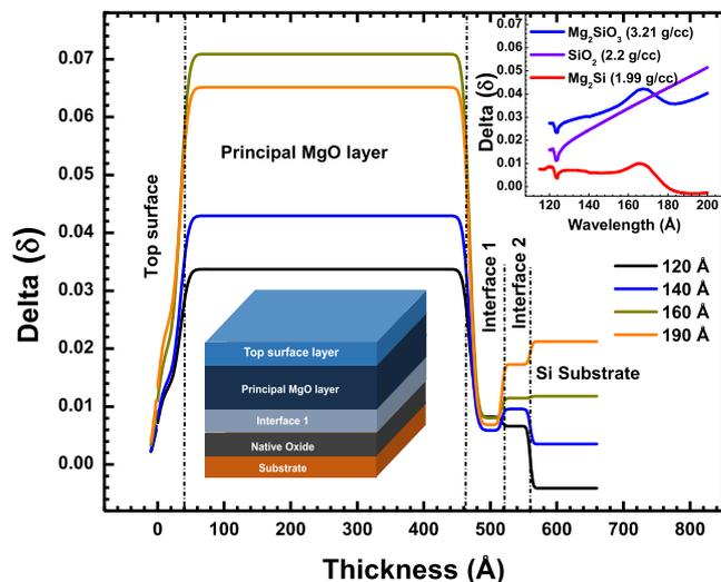
**FIGURE 3** In-depth optical density profile obtained from modelling the soft X-ray reflectivity data. Inset shows the Henke tabulated delta values in the wavelength range of 120-190 Å for bulk Mg<sub>2</sub>SiO<sub>3</sub>, SiO<sub>2</sub>, and Mg<sub>2</sub>Si
