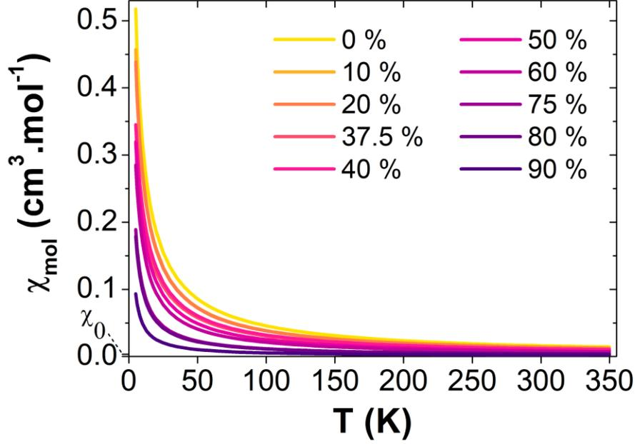
Figure 1: Molar susceptibility  $\chi_{\text{mol}}$  of  $\text{Gd}_{2(1-y)}\text{Ce}_{2y}\text{O}_2\text{S}$  powders measured by vibrating sample magnetometry. The average value of  $\chi_0$  is indicated on the ordinate axis. The y value is indicated in % in the legend. The applied field is 50 Oe.
