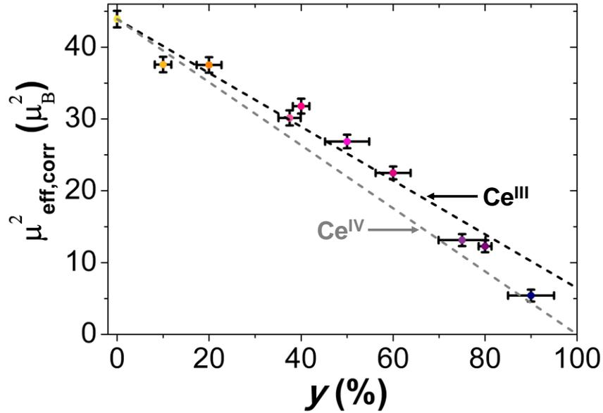
Figure 3: Experimental dependence of the square magnetic moments of  $\text{Gd}_{2(1-y)}\text{Ce}_{2y}\text{O}_2\text{S}$  nanoparticles on  $y$ . The raw values of magnetic susceptibility have been normalized by assuming that 30 wt% of the samples is made of oleate ligands. The broken black and gray lines indicate the dependence expected in the case of  $\text{Ce}^{\text{III}}$  or  $\text{Ce}^{\text{IV}}$  cations, respectively.
