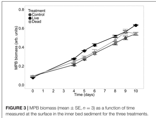
**FIGURE 3 |** MPB biomass (mean ± SE,  $n = 3$ ) as a function of time measured at the surface in the inner bed sediment for the three treatments.
