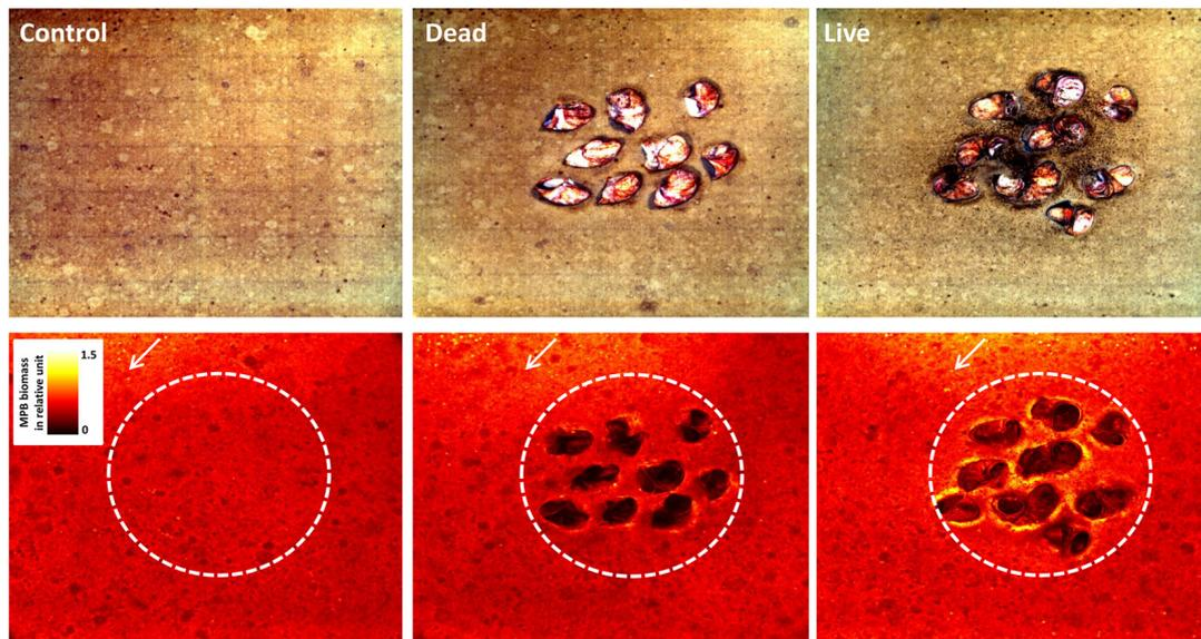
**FIGURE 2** | Top view of the sediment surface after 10 days in the experimental mesocosms with the control, dead and live treatments. Shown are examples of true-color images (top row) and the corresponding Microphytobenthos (MPB) biomass maps (in relative units; bottom row). White arrows indicate overlying seawater flow direction. Dashed circles represent the inner bed sediment area.
