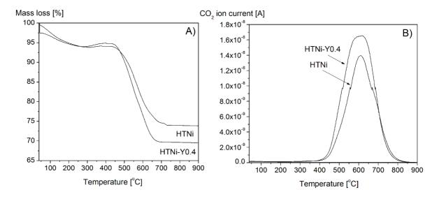
Fig. 9 TGA-MS over the spent catalyst (CH<sub>4</sub>/CO<sub>2</sub>/Ar=1/1/8, 700 °C for 5 h).
