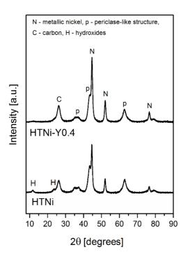
Fig. 8 XRD diffractograms of the spent catalysts (CH<sub>4</sub>/CO<sub>2</sub>/Ar=1/1/8, 700 °C for 5 h).
