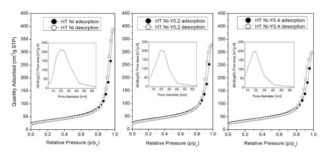
Fig. 1  $N_2$  adsorption/desorption isotherms and pore distribution for HTNi, HTNi-Y0.2 and HTNi-Y0.4 catalysts.
