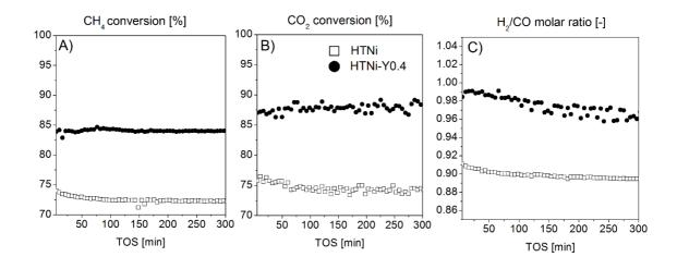
Fig. 6 Catalytic DRM tests at 700 °C (GHSV=20,000 h<sup>-1</sup>, CH<sub>4</sub>/CO<sub>2</sub>/Ar=1/1/8, total flow rate 100 cm<sup>3</sup>/min).
