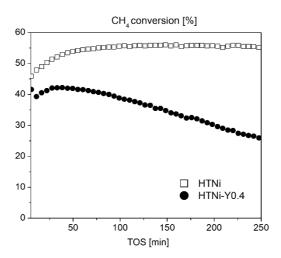
Fig. 7 Catalytic tests of direct methane decomposition as a function of temperature (GHSV=20,000 h<sup>-1</sup>, CH<sub>4</sub>/Ar=2/8, total flow rate 100 cm<sup>3</sup>/min).
