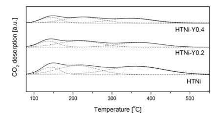
Fig. 4 TPD-CO<sub>2</sub> patterns recorded over the catalysts reduced at 900°C.
