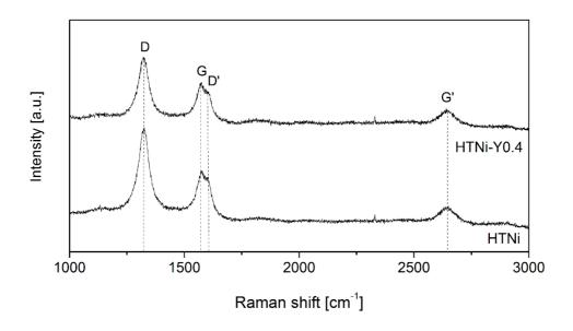
Fig. 10 Raman spectra over the spent catalysts (CH<sub>4</sub>/CO<sub>2</sub>/Ar=1/1/8, 700 °C for 5 h).
