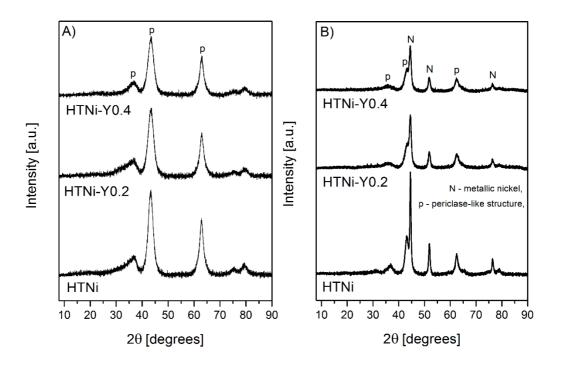
Fig. 2 XRD patterns of a) catalysts after calcination at 550 °C for 5 h, b) catalysts reduced in 5%  $H_2/Ar$  mixture at 900 °C for 1 h (GHSV= 20,000 h<sup>-1</sup>).
