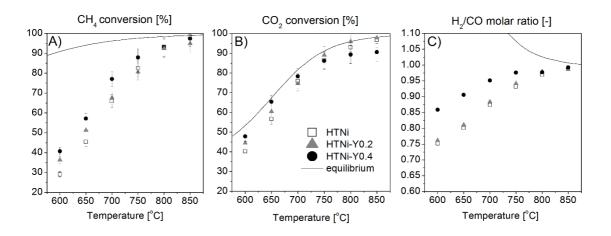
Fig. 5 Catalytic DRM tests as a function of temperature, steady-state measurements after 30 min at each temperature (GHSV=20,000 h<sup>-1</sup>, CH<sub>4</sub>/CO<sub>2</sub>/Ar=1/1/8, total flow rate 100 cm<sup>3</sup>/min<sup>-1</sup>).
