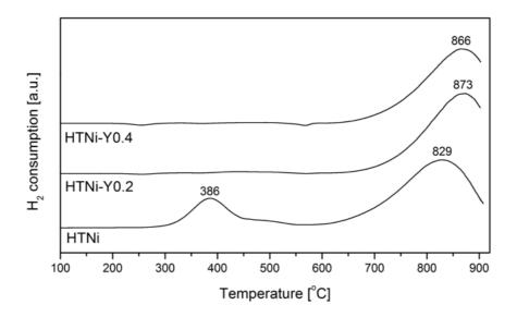
Fig. 3 TPR-H<sub>2</sub> profiles recorded over HTNi, HTNi-Y0.2 and HTNi-Y0.4.
