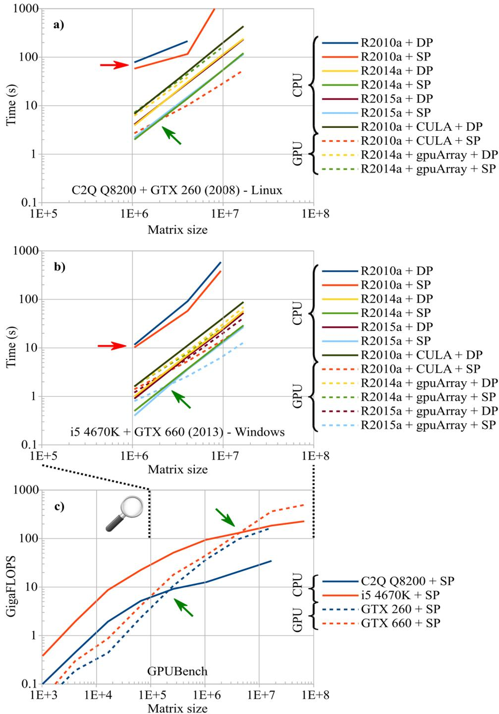
Figure 4: a) and b) Computation times for **SVD under Matlab**. Comparison of CPU and GPU times against matrix size for different Matlab versions. a) C2Q Q8200 + GTX 260 (2008). b) i5 4670K + GTX 660 (2013). c) SP performance against matrix size measured with GPUBench v1p7 under R2014a; the horizontal scale is larger than on a) and b). CPU and GPU times are drawn with plain and dashed lines, respectively. Red and green arrows indicate bad algorithm and CPU-GPU crossing, respectively.
