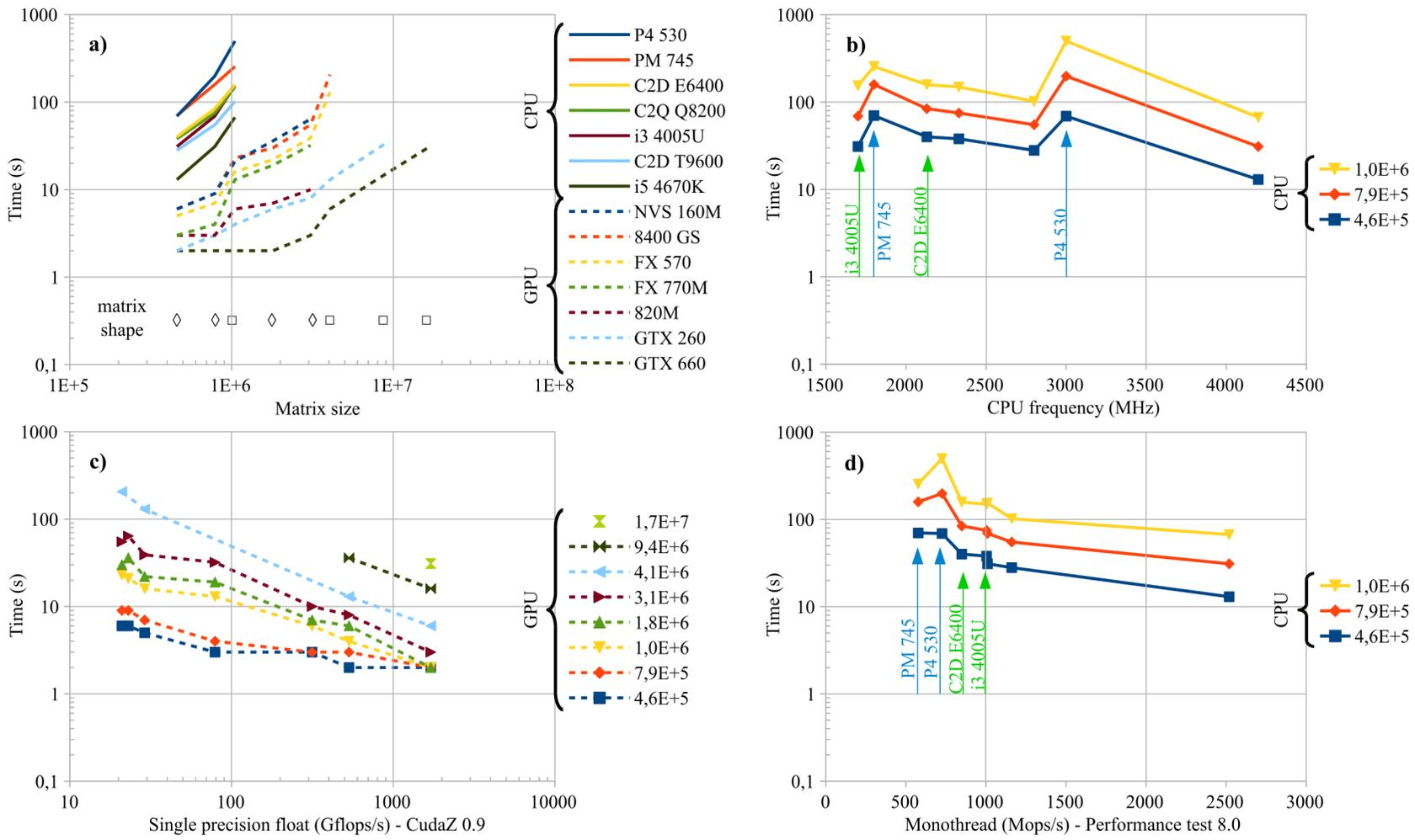
Figure 3: Computation times for **SVD under Java**. a) Comparison of CPU and GPU times against matrix size;  $\diamond$ : rectangular matrix;  $\square$ : square matrix. b) CPU times against CPU frequency. c) GPU times against single precision float performance. d) CPU times against monothread performance; light blue and light green arrows evidence CPU cache and CPU release year influence, respectively. CPU and GPU times are drawn with plain lines and dashed lines, respectively.
