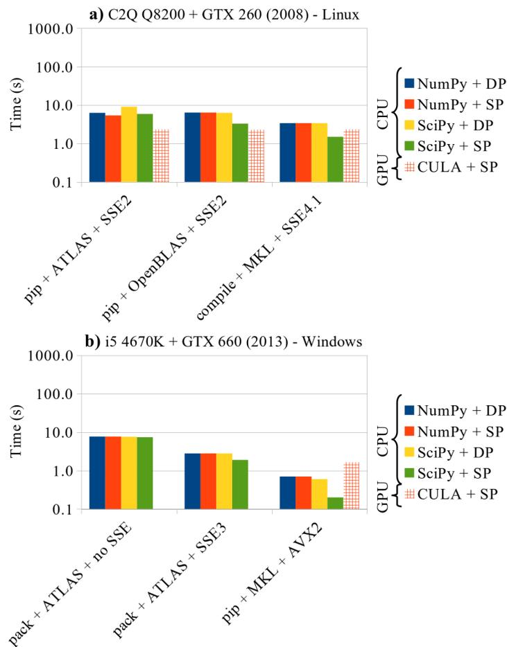
Figure 5: Computation times for **SVD under Python** with influence of libraries and hardware optimisations for a matrix size of  $1025 \times 1024 = 1.0e6$  points. a) C2Q Q8200 + GTX 260 (2008) under Linux. b) i5 4670K + GTX 660 (2013) under Windows.
