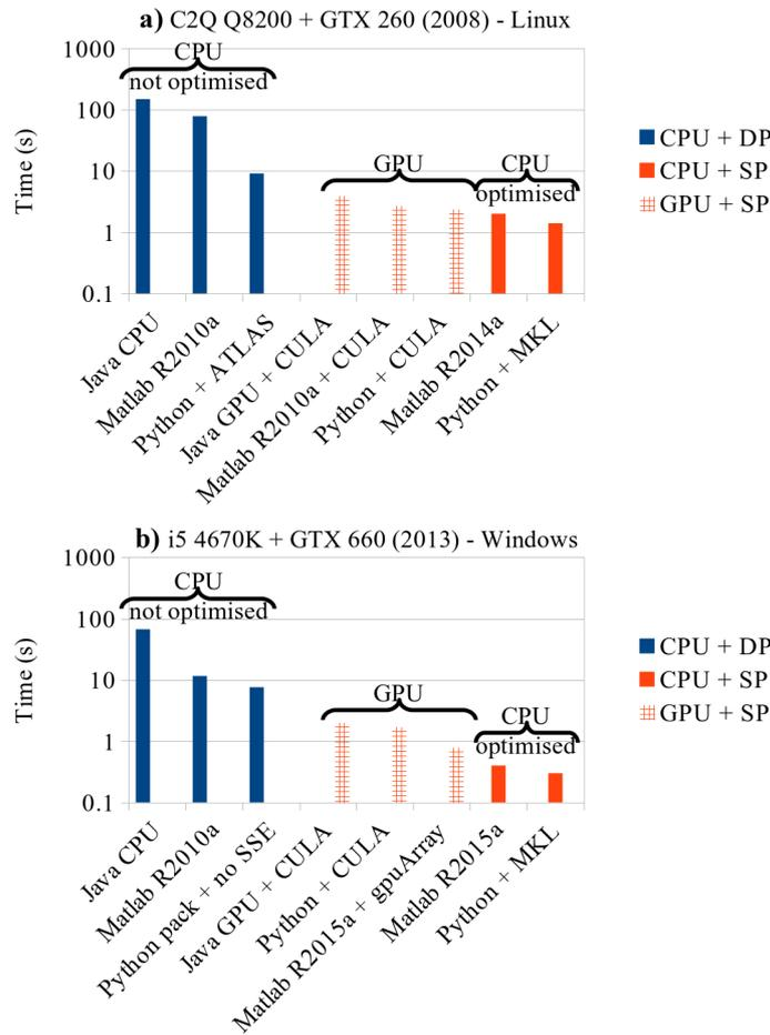
Figure 6: Comparison of **Java, Matlab and Python SVD** computation times for a matrix size of  $1025 \times 1024 = 1.0e6$  points, in logarithmic scale. a) C2Q Q8200 + GTX 260 (2008) under Linux. b) i5 4670K + GTX 660 (2013) under Windows.
