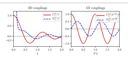
**Figure A1.** Collective couplings in 3D and 1D. Spatial dependence of the 3D (left) and 1D (right) coherent/incoherent coupling strengths as a function of distance between atoms as a function of the normalized distance  $\xi = k_0 d$ . Observe, that the 3D free space couplings decay with increasing distance, while the 1D contributions, shown for a single mode here, are periodic and of infinite range. Including several modes, finite ranges can be engineered as discussed below.
