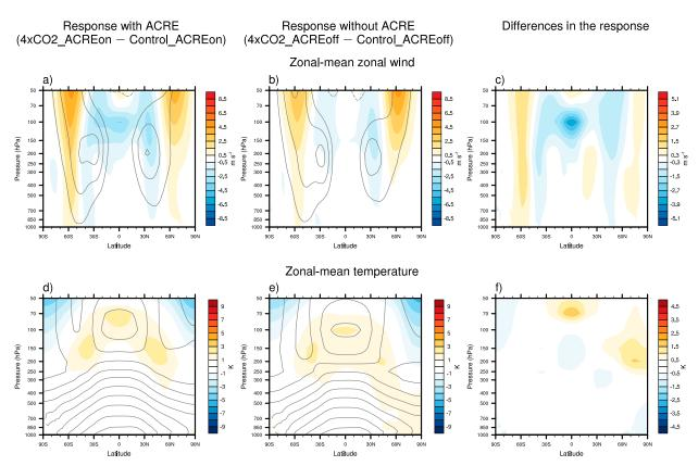
FIG. 3. As in Fig. 2, but for the circulation response (shading) to  $4 \times CO_2$  when ACRE are (left) on and (center) off, and (right) the differences between left and center columns. (a) Reproduction from Fig. 1b. (a)–(c) The zonal-mean zonal wind; (d)–(f) the zonal-mean temperature. Gray contours denote the corresponding climatology in (left) Control\_ACRE and (center) Control\_ACRE off.
