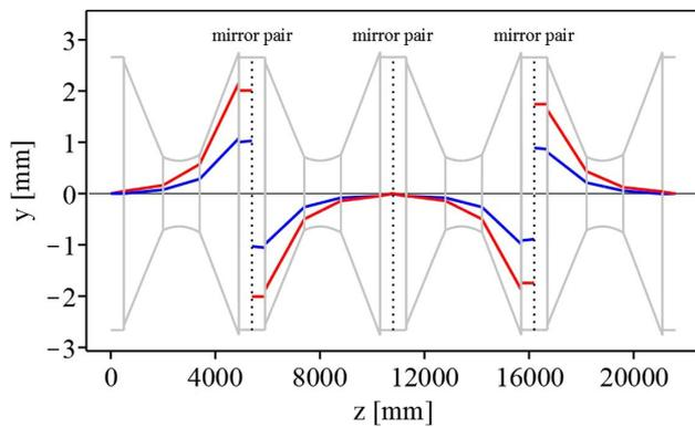
**Fig. 5.** Similar to Fig. 4, but for a multipass amplifier where M2 is replaced by a pair of  $45^\circ$  mirrors acting as a vertical retro-reflector. The vertical dotted lines indicate the position of the retro-reflector. The excursion is shown only for the vertical component. The horizontal component is not affected by the vertical retro-reflector, so that it follows the evolution shown in Fig. 4.
