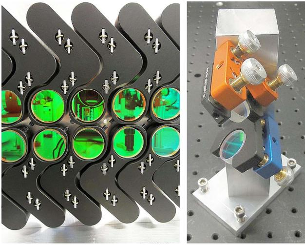
**Fig. 3.** (Right) Photo of the custom-designed mirror array with L-shaped adjustable mirror holders. The horizontal spacing between the 25 mm mirrors is 31 mm. (Left) Picture of the pair of 45° mirrors acting as a vertical retro-reflector, which can assume the functionality of the mirror M2 in Fig. 2.
