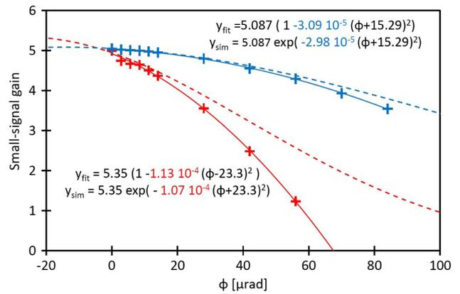
**Fig. 8.** Small signal gain versus disk tilt in vertical direction. The red points were measured for the multipass amplifier in Fig. 2 with a simple M2 mirror. The blue points have been obtained from the same amplifier but with M2 replaced by a vertical retro-reflector. The measurements have been fitted with parabolic functions (solid lines). The dashed curves represent the predictions from Eqs. (16) and (17) normalized to match the maxima of the parabolic fits.
