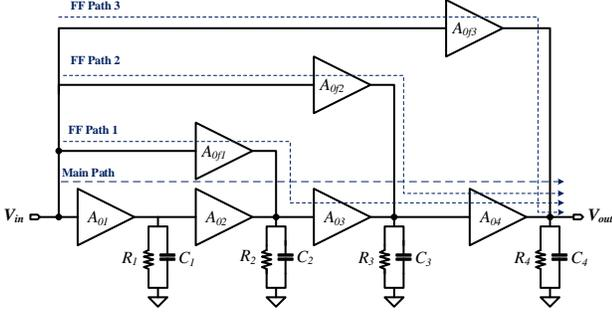
Figure 4: System-level diagram of the 4<sup>th</sup>-order FF-compensated op-amp
