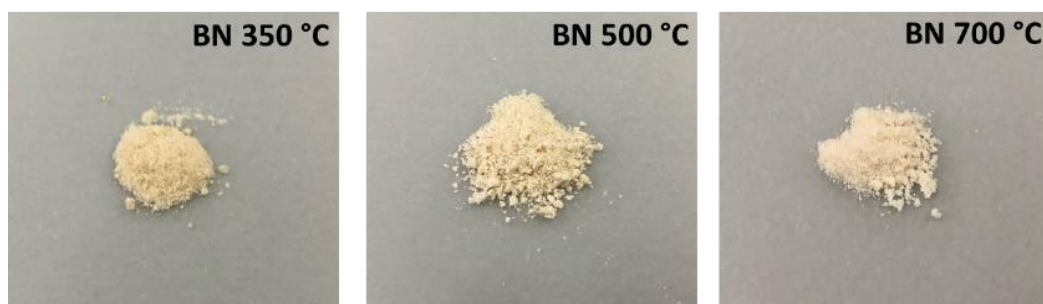
Figure S10. Powders acquired by pyrolysis of AB at varying temperatures.
