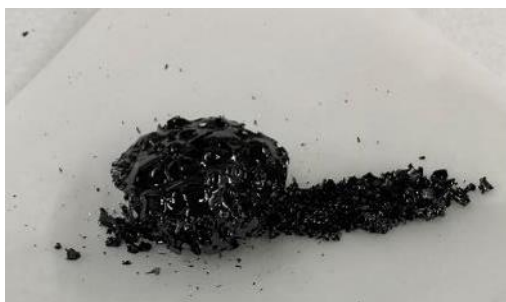
Figure S8. Picture of 2 g of BN Pyr700 made in a single synthesis before grinding.
