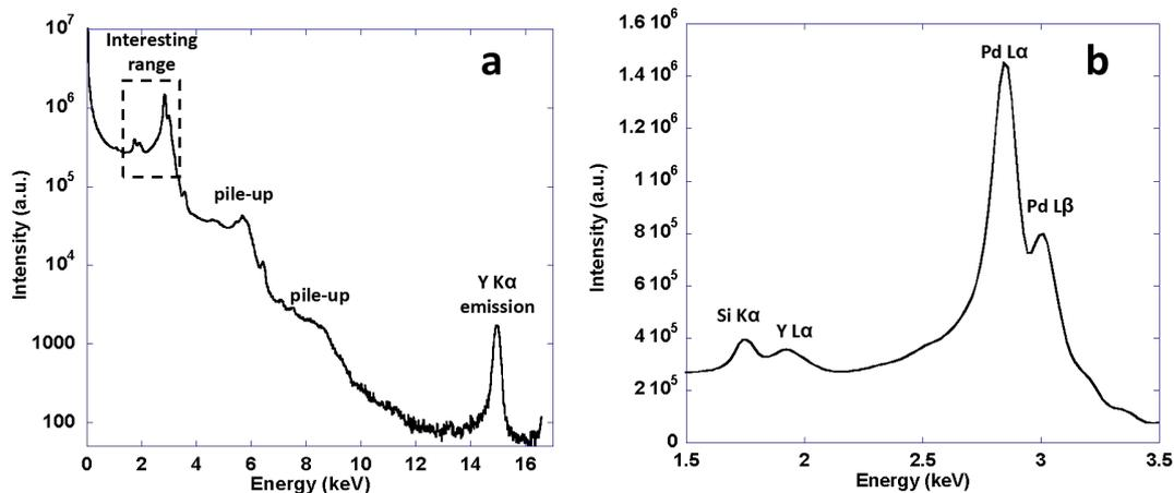
Fig. 2. Spectrum of  $\text{B}_4\text{C}(2.5 \text{ nm})/[\text{Pd}(2 \text{ nm})/\text{B}_4\text{C}(2 \text{ nm})/\text{Y}(2 \text{ nm})]_{\times 40}/\text{Si}$  multilayer: a) overview, intensity in log scale; b) zoomed range of interest, intensity in linear scale.
