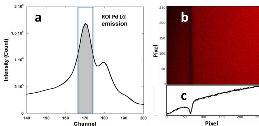
Fig. 3. a) Selection of the ROI for Pd  $L\alpha$  emission; for the case already depicted in Fig. 1: b) image of the intensity of X-ray emission, of which the energy is in the ROI; c) Kossel curve depicted by integrating the X-ray emission intensity along the vertical pixel.
