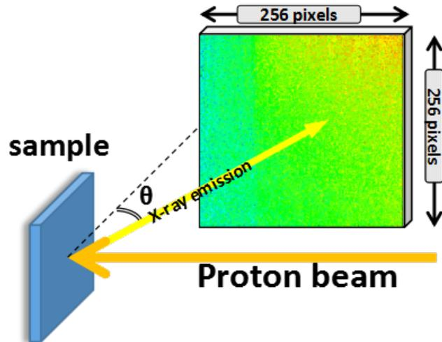
Fig. 1. Geometry of the experimental setup.  $\theta$  is the detection angle. The presented experimental image is the spatial distribution of total X-ray intensity on the detector array for  $\text{B}_4\text{C}(2.5 \text{ nm})/[\text{Pd}(2 \text{ nm})/\text{B}_4\text{C}(2 \text{ nm})/\text{Y}(2 \text{ nm})]_{\times 40}/\text{Si}$  multilayer irradiated as described in the text.
