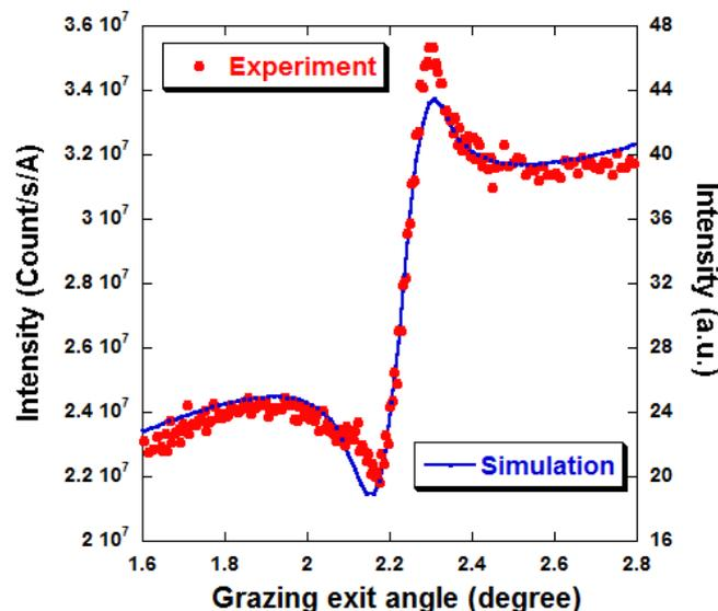
Fig. 7. Comparison between experimental result and simulation of the PIXE-Kossel curves of the sample  $B_4C(2.5\text{ nm})/[B_4C(1\text{ nm})/Pd(2\text{ nm})/B_4C(1\text{ nm})/Y(2\text{ nm})]_{\times 20}/Si$ .
