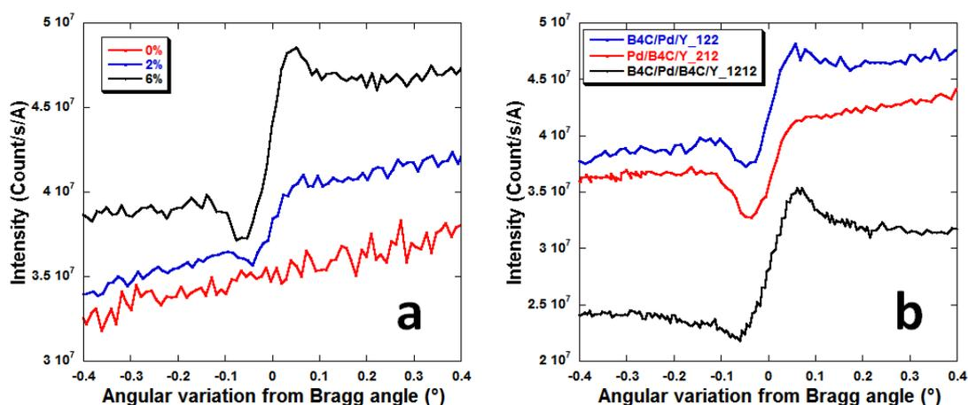
Fig. 6. Kossel curves for Pd  $L\alpha$  emission of all measured samples. a) series of samples fabricated with different concentration of  $N_2$  in the sputtering gas; b) series of samples with  $B_4C$  barrier layers at one given interface or at both interfaces. For this latter series, the name of the samples refers both to the order of the layers within the period and to the thickness (in nm) of the individual layers.
