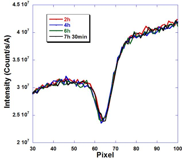
Fig. 4. Non-damaging test of the sample  $B_4C(2.5 \text{ nm})/[Pd(2 \text{ nm})/B_4C(2 \text{ nm})/Y(2 \text{ nm})]_{\times 40}/Si$ .
