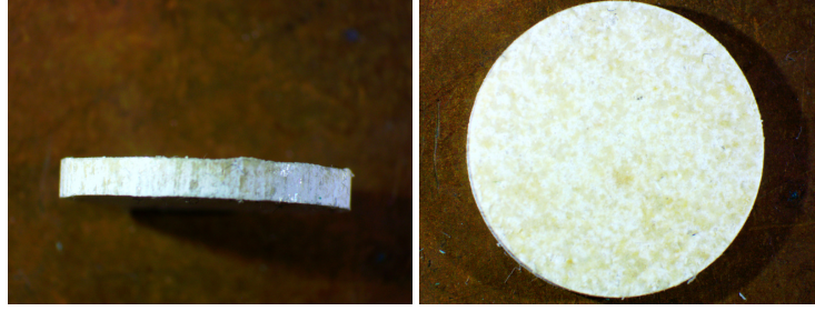
Figure 1: Photographs of a polycrystalline RTO pellet before electrode deposition. The diameter is 15mm. The differences in color are presumably due to different hydration degrees of RTO.
