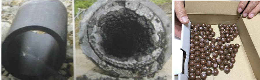
Figure 1: Unwanted effect of scale and the device studied here to cure it
