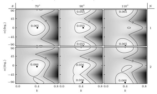
Figure 5: Growth rate  $\sigma_{\Sigma}$  as a function of the wavenumber k and the orientation  $\alpha$  of the bed perturbation for  $u_*/u_{th} = 5$  and different values of the divergence angle  $\theta$  (columns) and the transport ratio N (rows). Black dots: most unstable mode ( $\alpha_{sat}, k_{sat}$ ).
