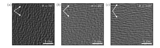
Figure 12: Photographs of the dune pattern in the experiment across the transition from transverse to longitudinal orientations, starting from a flat bed, for  $V/V_{th} = 1.4$ . Flow directions are shown with arrows. From left to right, the pictures have been taken after 30, 32, and 30 blows, respectively
