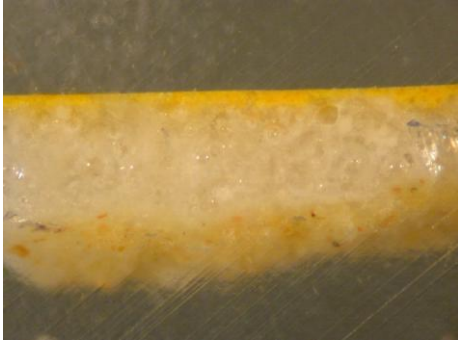
Fig. S5: cross-section optical microscopy image of a yellow glaze from the Palcio Gotico large room : 10 \mu\text{m} yellow layer and 160-190 \mu\text{m} white layer on the body
