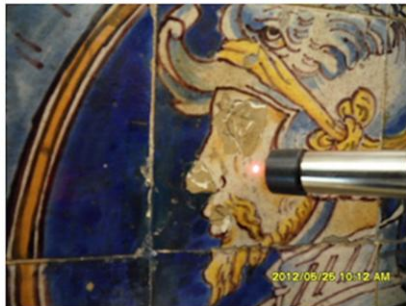
Fig. 2: Palacio Gotico (a) view of the large room with the team at work on the left; (b) tiles showing a portrait of Carlos Quinto ; the tip of the X ray detector (2 cm diameter) is next to the measurement point indicated by a laser impact; (c) tiles in the small room. Yellow, orange and blue colors can be seen.
