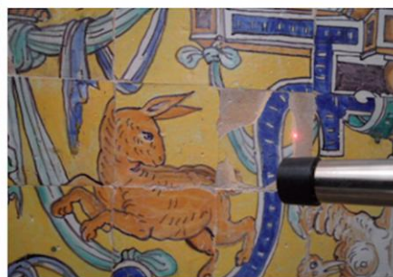
Fig. 2: Palacio Gotico (a) view of the large room with the team at work on the left; (b) tiles showing a portrait of Carlos Quinto ; the tip of the X ray detector (2 cm diameter) is next to the measurement point indicated by a laser impact; (c) tiles in the small room. Yellow, orange and blue colors can be seen.
