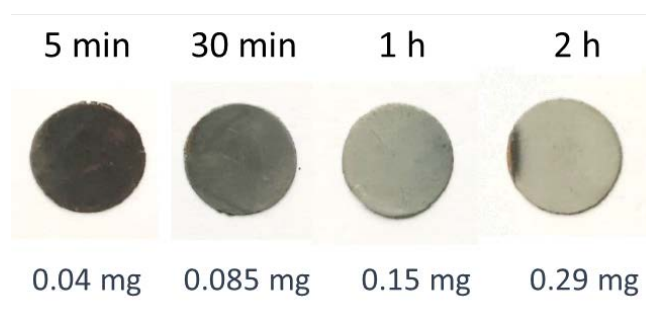
Figure S4. Images of the electrodes after different deposition time on Cu substrate.
