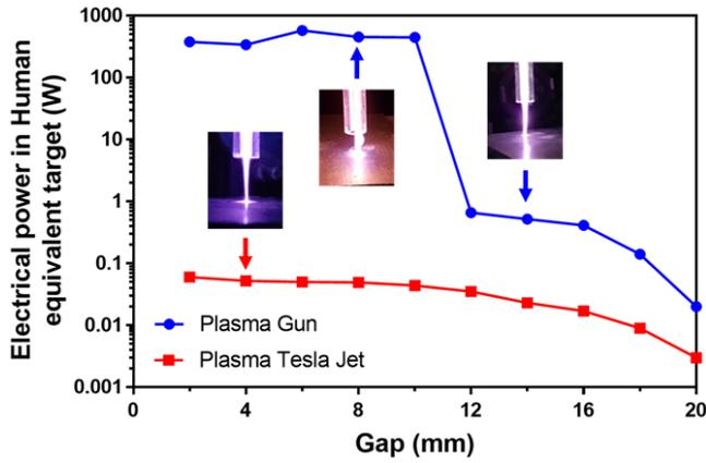
**Figure 13.** EEHB target power as a function of the gap for PG and PTJ devices. Experimental conditions:  $V_0 = 7$  kV, helium flow rate = 1000 sccm, repetition frequency = 30 kHz and duty cycle = 14%. No measurement capacitor  $C_{m1}$  is present in the electrical circuit.
