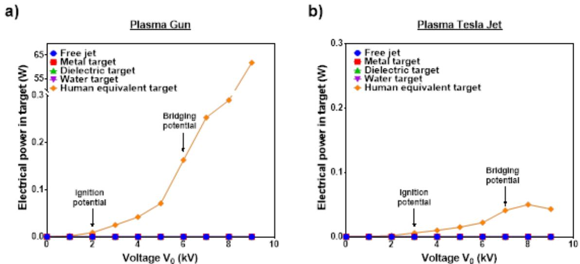
**Figure 6.** Comparison of electrical power deposited in targets using (a) PG and (b) PTJ. Experimental conditions: helium flow rate = 1000 sccm, repetition frequency = 30 kHz, duty cycle = 14% and gap = 10 mm.
