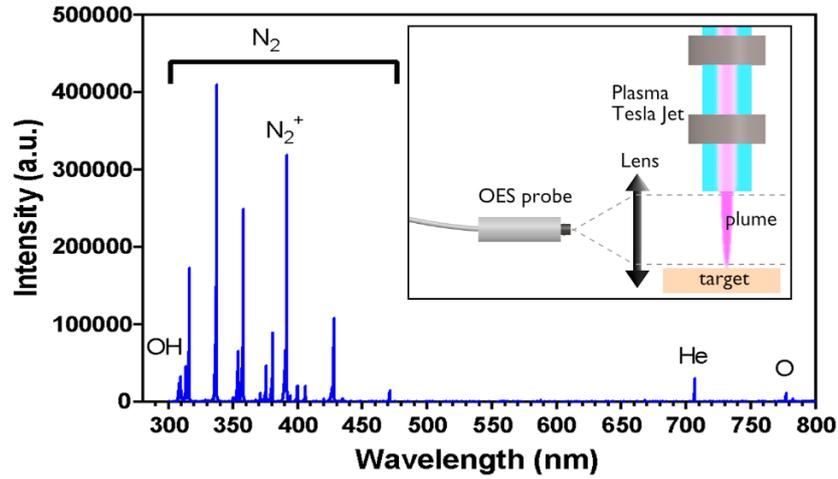
**Figure 8.** Optical emission spectra of the plumes generated by PG and PTJ. The two spectra overlap whatever the APPJ with/without target interaction. The inset indicates how plasma emission is collected: along the jet axis (i.e. side-on) without spatial resolution.
