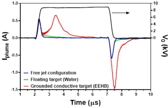
**Figure 12.** Influence of targets on instantaneous current in PG plume. Experimental conditions: Voltage 9 kV, helium flow 1000 sccm, frequency 30 kHz and duty cycle 14%. Voltage waveform is indicated in solid black line.
