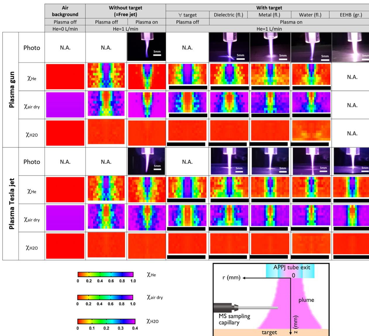
**Figure 7.** 2D profiles of gas molar fractions for PG and PTJ with/without target interaction. Experimental conditions: Voltage 7 kV, helium flow rate = 1000 sccm, frequency = 30 kHz, duty cycle = 14% (electrical plasma power = 12 W) and gap = 10 mm. The inset indicates how the MS capillary is positioned for perform the mapping.
