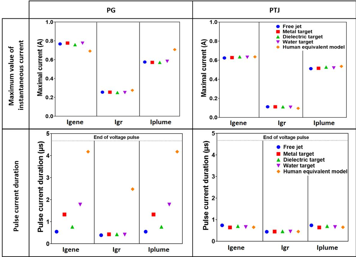
**Figure 5.** Maximum values of current and pulse current durations for PG and PTJ with/without target interaction. Experimental conditions:  $V_0 = 9$  kV, helium flow rate = 1000 sccm, repetition frequency = 30 kHz, duty cycle = 14%, gap = 10 mm. The error bars are not visible due to the high reproducibility of the measurements ( $<2\%$ ).
