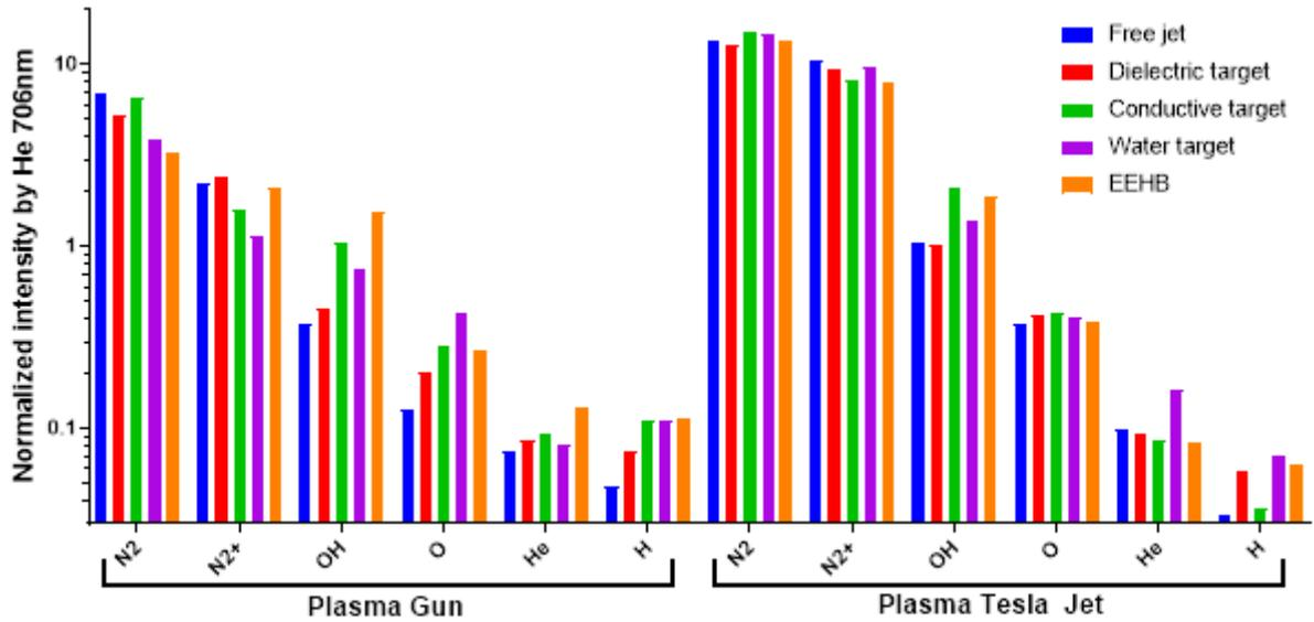
**Figure 9.** Normalized intensity of OES lines and bands using PG and PTJ with/without target.  $V_0 = 7$  kV, i.e.  $P_{\text{plasma}} = 12$  W for all configurations except for the PG-EEHB configuration where  $P_{\text{plasma}} = 26$  W).
