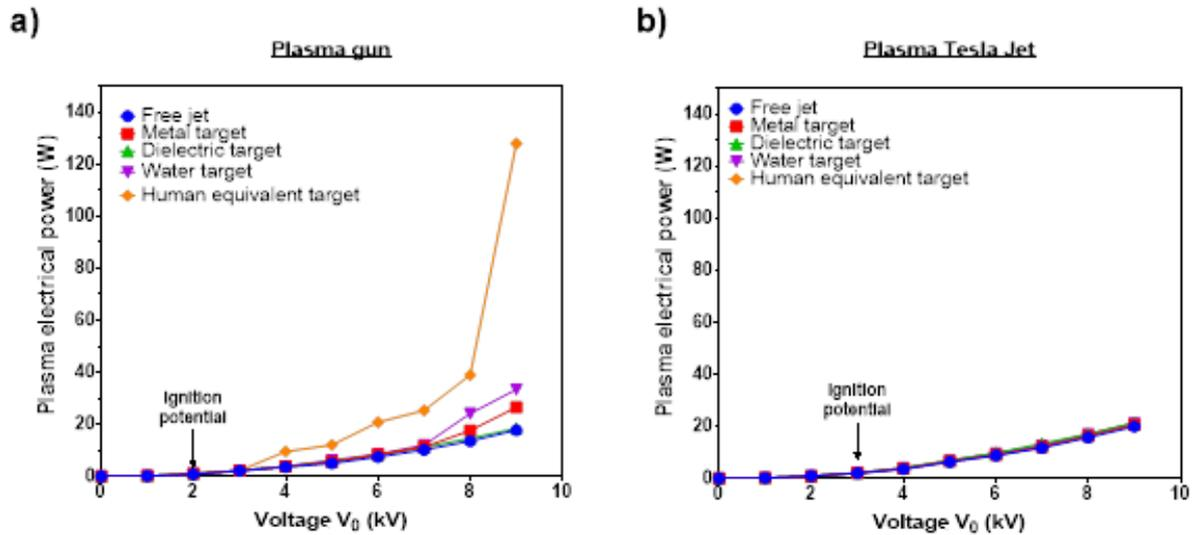
**Figure 4.** Electrical plasma power per pulse as a function of the plasma voltage considering free jet or jet-target configurations for (a) PG and (b) PTJ. Experimental conditions: helium flow rate = 1000 sccm, frequency = 30 kHz, duty cycle = 14% and gap = 10 mm.
