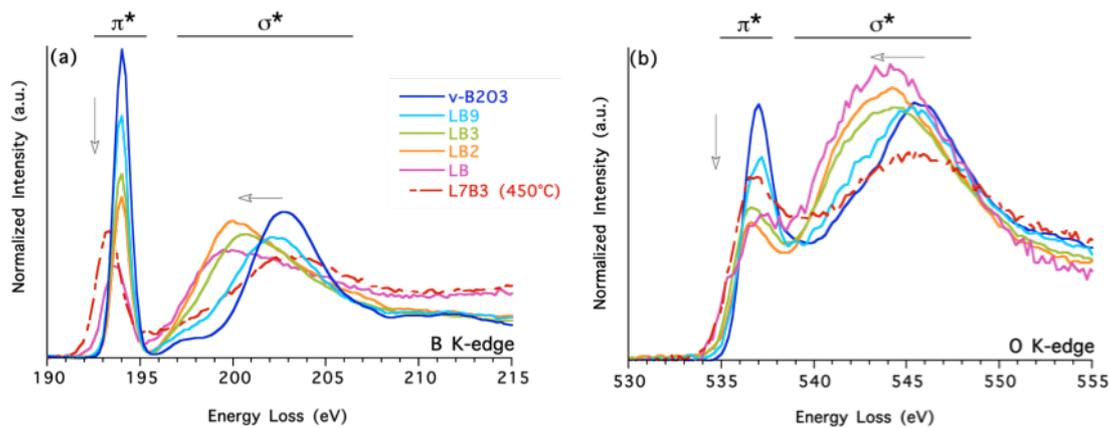
**Fig. 1:** (a) Effect of  $\text{Li}_2\text{O}$  content on both (a) B  $K$ -edge and (b) O  $K$ -edge NRIXS spectra of six lithium borate glasses:  $v\text{-B}_2\text{O}_3$  (blue), LB9 (cyan), LB3 (green), LB2 (orange), LB (pink) and L7B3 (red). All the spectra were obtained at room temperature except those for L7B3 (measured at  $450^\circ\text{C}$  for both B and O  $K$ -edges) and for LB3 (measured at  $250^\circ\text{C}$  for O  $K$ -edge only).
