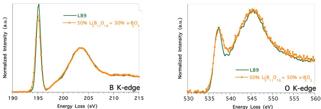
**Fig. 5:** B *K*-edge (left) and O *K*-edge (right) NRIXS spectra of the LB9 glass (green) accompanied with the linear combination of  $v\text{-B}_2\text{O}_3$  and  $\text{Li}_3\text{B}_{11}\text{O}_{18}$  spectra (orange).
