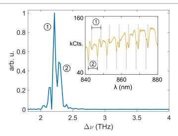
**Figure 7.** Blue: Fourier transform of experimental transmission spectrum. Inset yellow: zoom of the figure 6(b). Two different sets of peaks can be seen. The corresponding  $\Delta v_{\rm FSR}$  are 2.21 and 2.28 THz (peaks location in the blue curve). This splitting corresponds to different polarization modes undergoing birefringence along the propagation in the structure.
