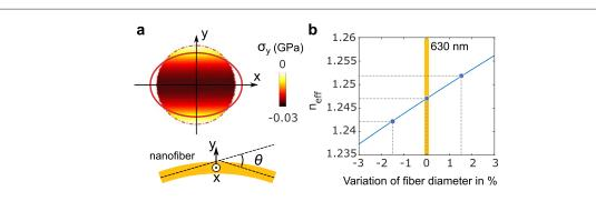
**Figure 8.** Brazier effect on a bent optical fiber. (a) Schematic of the fiber cross-section (x–y plane) ovalization.  $\sigma_y$  is the y component of the bending induced stress, represented with the color scale within the fiber cross-section.  $\theta$  is the angle of rotation of the fiber ends. (b) Relative refractive index variation as a function of the fiber diameter change in percent compared with an initial diameter of 630 nm.
