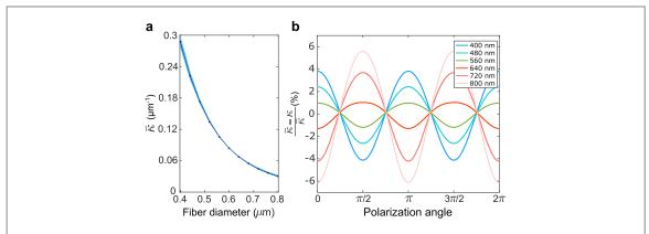
**Figure 4.** (a) Coupling coefficient  $\kappa$  (at 800 nm) between nanofibers with varying diameter and averaged over the polarization degree of freedom. The colored area refers to the amplitude of the variation with the polarization. (b) Relative change of the coupling coefficient as a function of the polarization angle with a fiber diameter varying from 500 to 900 nm.
