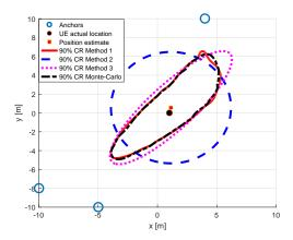
Figure 3 - 90% confidence regions, obtained by the three methods, and assessed by a Monte-Carlo calculation. The standard deviations are 5, 5 and 15°, respectively.
