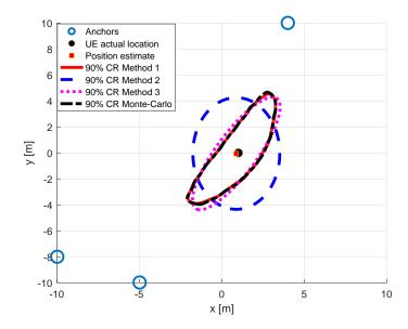
Figure 1 - 90% confidence regions, obtained by the three methods, and assessed by a Monte-Carlo calculation. The three AoA's are defined with a 5° standard deviation.
