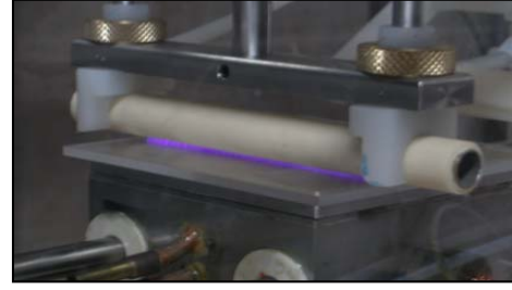
Fig. 1. (a) Schematics of the DBD used for the growth of NC thin film by nebulization of a colloidal suspension of Gr/HMDSO ( 360.8 \mu\text{l} \cdot \text{min}^{-1} in 8 slpm of argon), (b) Picture showing the plasma discharge.
