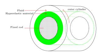
Fig. 1: A fluid-structure system inside a rotating cylinder with a fixed rod in its center. Sketch of the system.
