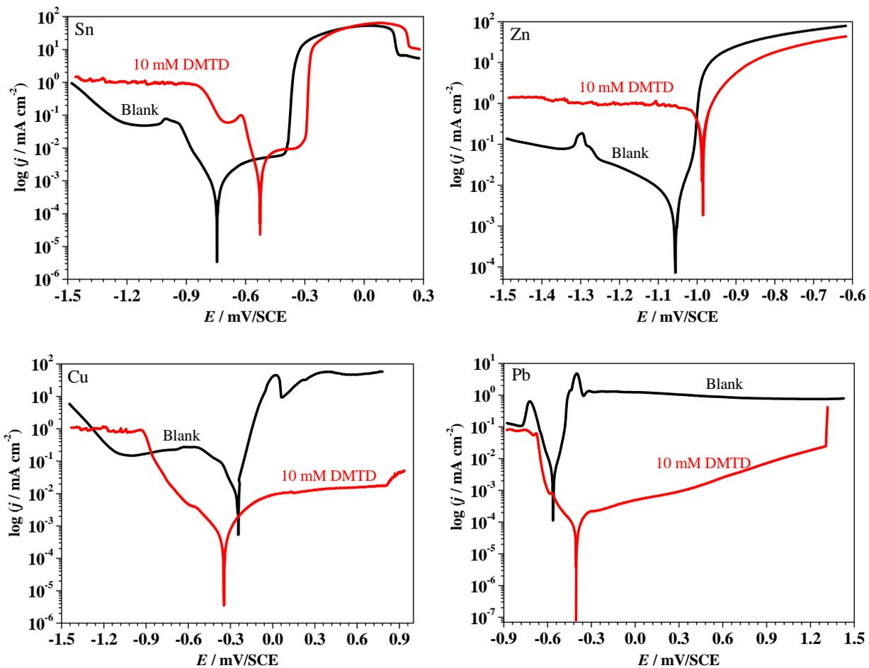
Figure 8: Effect of 10 mM DMTD on the electrode kinetics of Cu, Sn, Pb and Zn electrodes in 30 g L<sup>-1</sup> NaCl after one hour of immersion; stationary electrodes at 20 °C.
