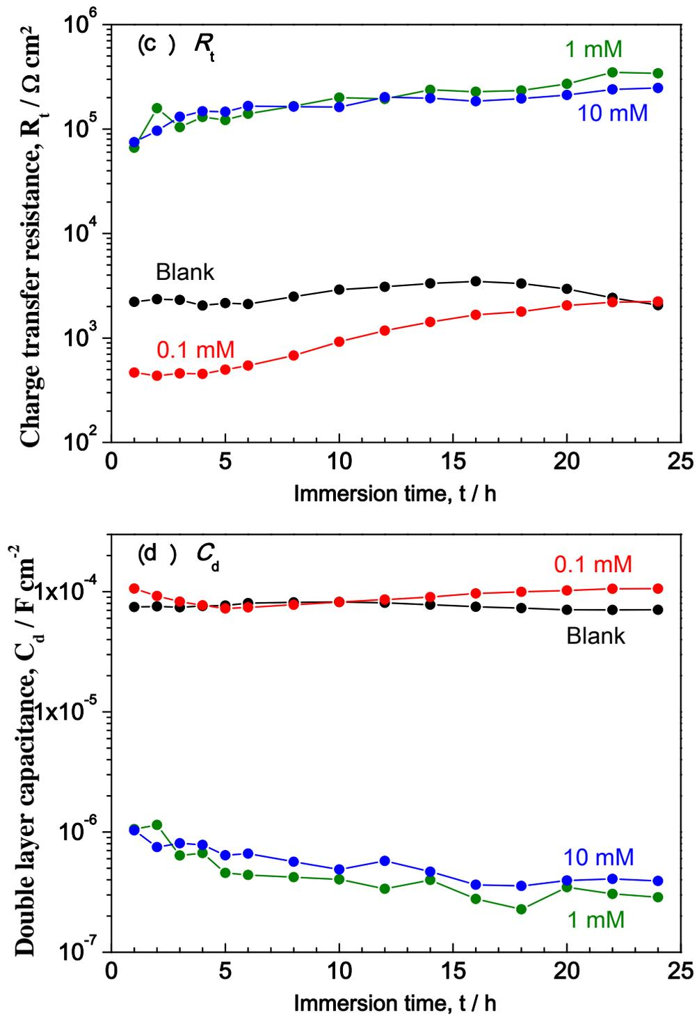
Figure 11:  $R_f$  (a),  $C_f$  (b),  $R_t$  (c) and  $C_d$  (d) change as a function of immersion time for bronze / 30 g L<sup>-1</sup> NaCl + DMTD at different concentrations; stationary electrode at 20 °C.
