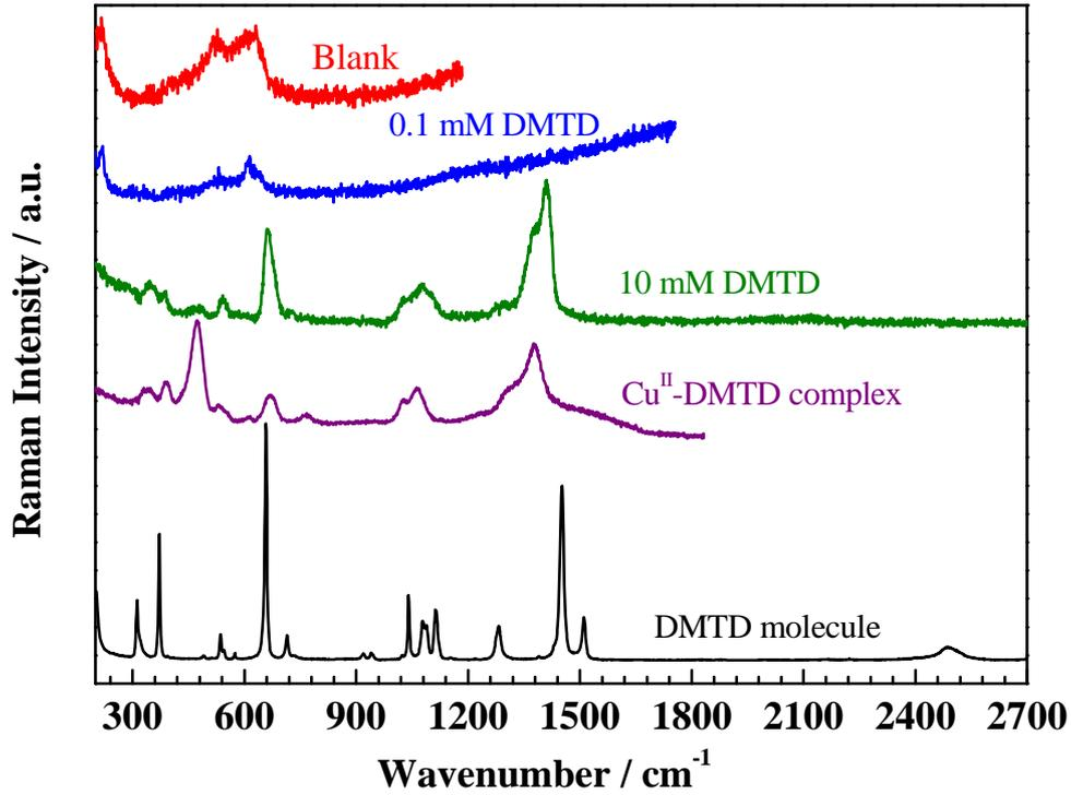
Figure 2: Raman spectra collected on DMTD molecule, Cu<sup>II</sup>-DMTD complex and on bronze electrode after 24 h immersion in 30 g L<sup>-1</sup> NaCl without or with 0.1 mM or 10 mM DMTD.
