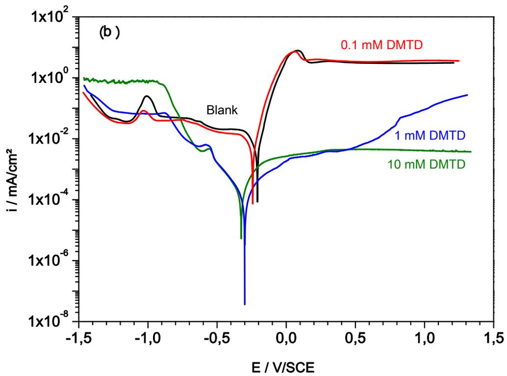
Figure 7: Open circuit potential plots (a) for bronze during one hour exposure time in  $30 \text{ g L}^{-1}$  NaCl without or with different concentrations of DMTD and polarization plots (b) after exposure; stationary electrode at  $20 \text{ }^\circ\text{C}$ .
