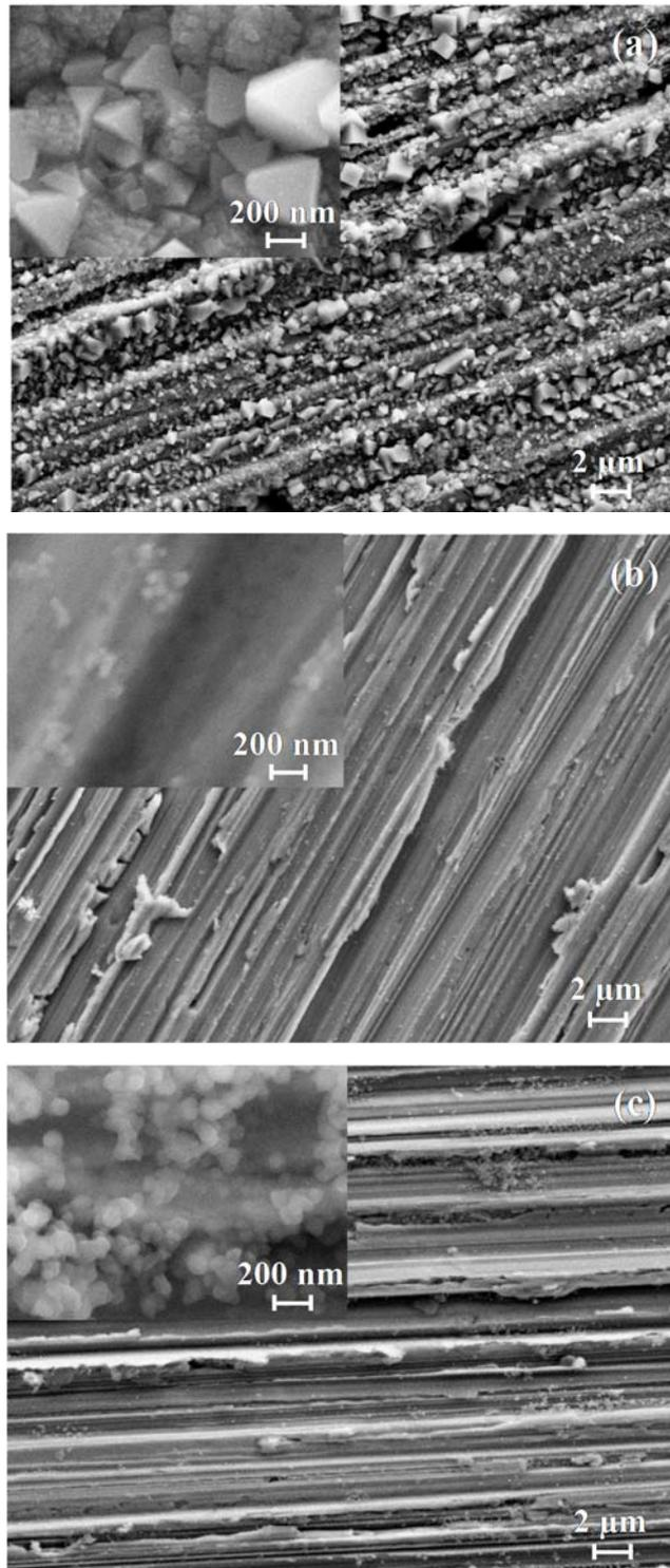
Figure 1: SEM images of bronze surface after 24 h immersion time in 30 g L<sup>-1</sup> NaCl with 0.1 mM (a), 1 mM (b) and 10 mM DMTD (c).
