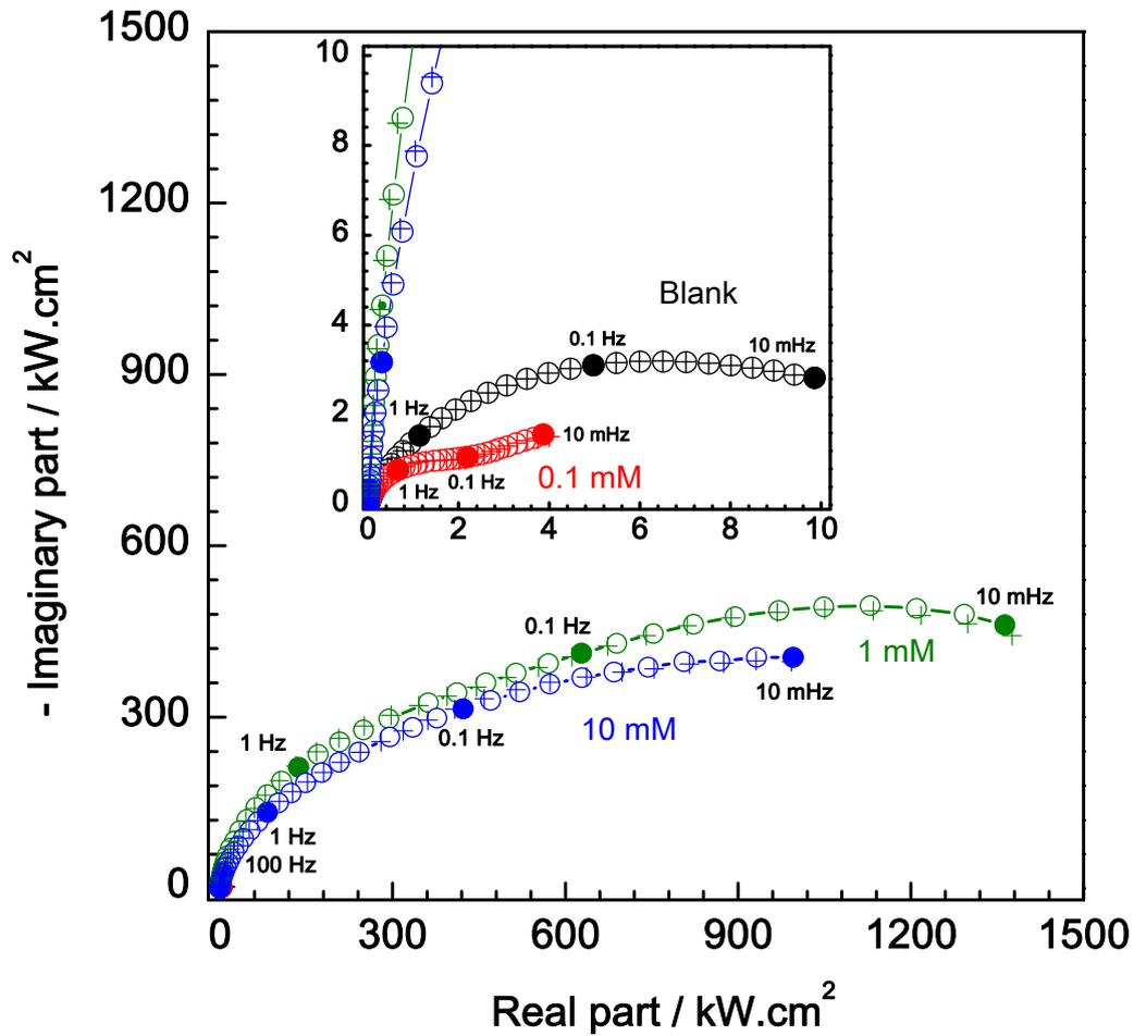
Figure 9: Nyquist diagrams of bronze after 24 hours exposure time in 30 g L<sup>-1</sup> NaCl + DMTD at different concentrations; stationary electrode at 20 °C.
