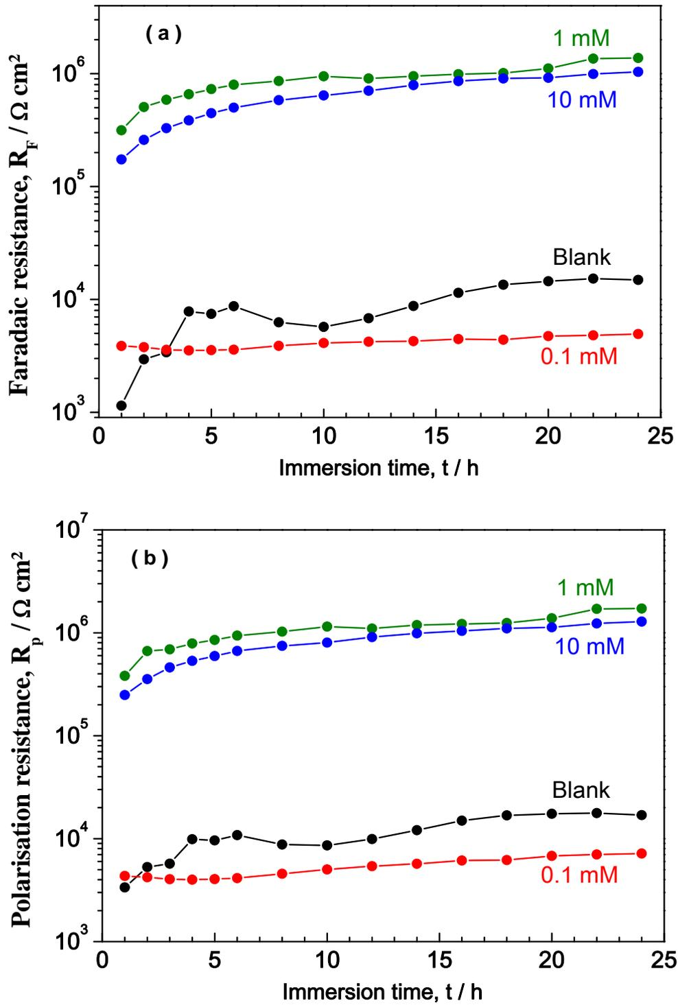
Figure 12:  $R_F$  (a) and  $R_p$  (b) change as a function of immersion time in bronze / 30 g L<sup>-1</sup> NaCl + DMTD at different concentrations; stationary electrode at 20 °C.
