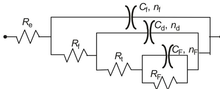
Figure 10: Electrical equivalent circuit to reproduce experimental impedance spectra for bronze electrode in NaCl solution without or with DMTD.
