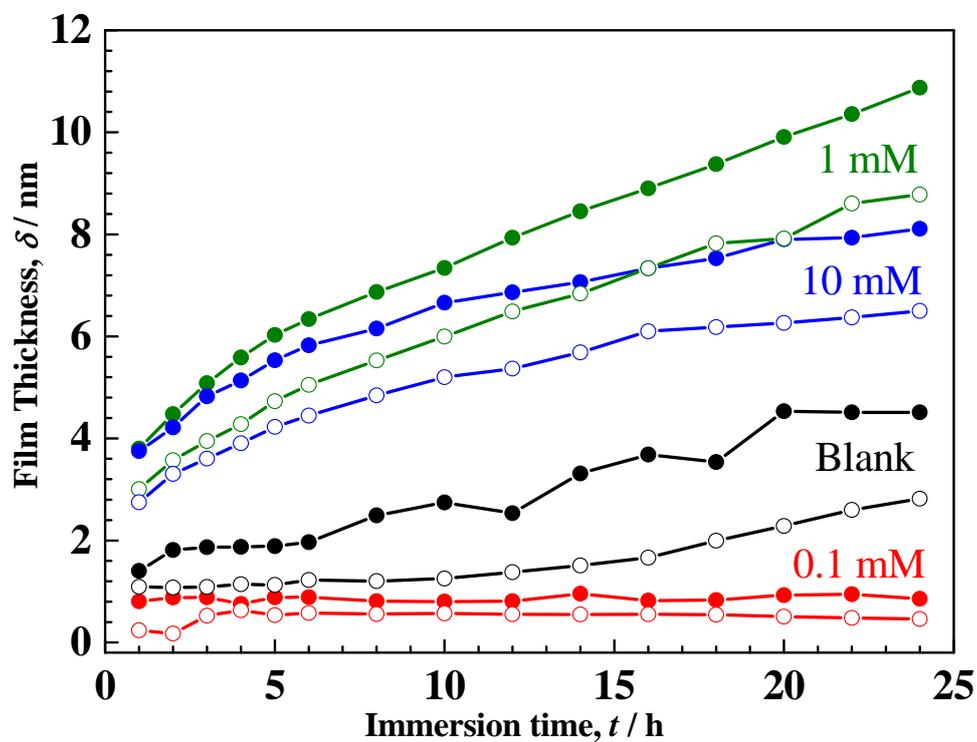
Figure 13: Thickness of films formed on bronze, determined from  $C_\infty$  (full circles) and  $C_f$  (open circles), as a function of immersion time in  $30 \text{ g L}^{-1} \text{ NaCl} + \text{DMTD}$  at different concentrations; stationary electrode at  $20 \text{ }^\circ\text{C}$ .
