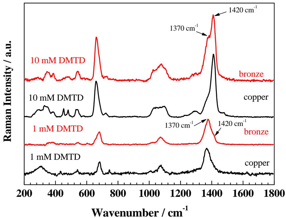
Figure 3: Raman spectra collected on bronze and copper electrodes after 24 h immersion in 30 g L<sup>-1</sup> NaCl with 1 mM or 10 mM DMTD.
