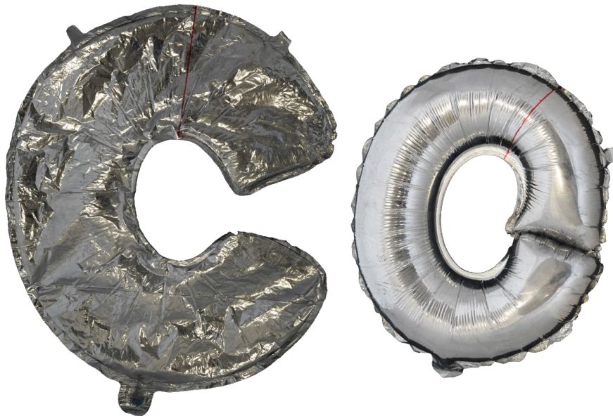
Fig. S3. Pictures of the same commercial mylar balloon before (left) and after (right) inflation. The letter, which looks like a "C" in the rest state, coils onto an "O" upon inflation.
