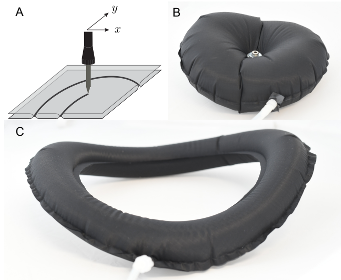
Fig. 1. Flat sealed inflatables. (A) Heat sealing of two sheets together along a desired path using a soldering iron mounted on an XY-plotter. (B) Photograph of an experimental realization of inflating an annulus of inner radius R and width w , with R/w \rightarrow 0 . Wrinkles appear and two diametrically opposed kinks are observed. (C) For R/w \gg 1 the inflated structure buckles smoothly out of plane. Both structures are made of Thermo-Plastic-polyUrethane coated nylon fabric.
