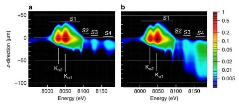
Fig. 8 Effect of hot electron population. Synthetic spatially resolved spectra employing the same plasma parameters but different multiplication factors of the hot electron fraction, **a** hot electron populations from the ab initio simulation, **b** hot electron fraction decreased by a factor of 10
