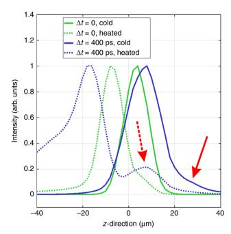
**Fig. 7** Effect of temporal delay on the X-ray emission. Simulated spatial distribution of  $K_{\alpha}$ -radiation emitted from cold and heated plasma regions. The electron distribution has a Gaussian profile delayed by  $\Delta t=0$  or 400 ps versus the laser maximum
