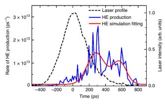
**Fig. 5** Temporal evolution of hot electrons. The production rate of hot electrons is obtained from the hydrodynamic simulation (blue); red line shows a two-parameter low resolution fit. The black dashed line shows the laser temporal profile for comparison
