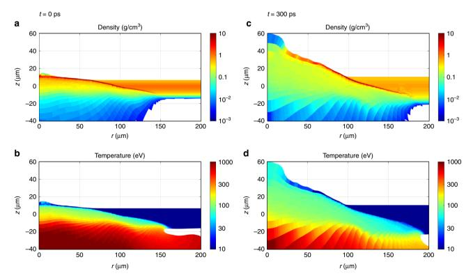
**Fig. 4** Plasma profiles from the hydrodynamic simulation. 2D distributions (r, z) of the plasma mass density  $(\mathbf{a}, \mathbf{c})$  and temperature  $(\mathbf{b}, \mathbf{d})$  on logarithmic scale obtained from the hydrodynamic simulation at the time of the laser pulse maximum (t = 0)  $(\mathbf{a}, \mathbf{b})$  and at the end of the laser pulse, t = 300 ps  $(\mathbf{c}, \mathbf{d})$
