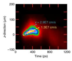
**Fig. 10** Plasma expansion visualized by X-ray streak camera. The laser is coming from below, the volume of the maximum emission moves with a velocity of  $1.3 \times 10^7$  cm/s
