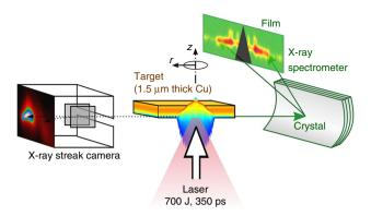
**Fig. 1** Experimental setup. The laser beam ( $\lambda=1.315~\mu m$ ,  $I=4.55\times 10^{15}~W cm^{-2}$ ) irradiates a 1.5-μm-thick Cu foil at normal incidence. The Cu K-shell emission is observed by spatially resolving crystal spectrometer and a temporally resolving streak camera
