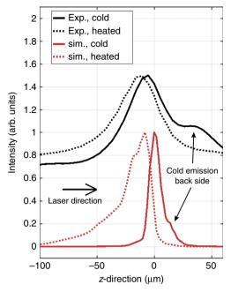
**Fig. 6** Spatial profiles of X-ray emission from plasma. Comparison of axial distributions of cold and heated  $K_{\alpha}\text{-emission}$  obtained from the experiment and simulations
