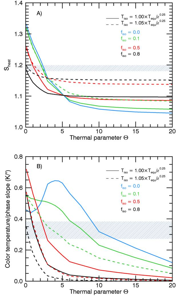
**Fig. 10.** Superheating factor  $S_{\text{heat}}$  (A) and phase linear dependence of the color temperature (B) from the thermal model parameterized by the thermal parameter  $\Theta$ , the optical depth contribution of isothermal particles  $f_{\text{iso}}$ , and their physical temperature  $T_{\text{iso}}$ . The shaded areas correspond to the measurements in the coma of 67P.
