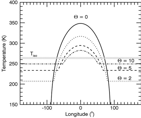
**Fig. 9.** Diurnal temperature profiles at equator of the modeled particles for different values of the thermal parameter  $\Theta$ . The subsolar point is at zero latitude and longitude. For large  $\Theta$ , the temperature reaches the constant isothermal value  $T_{\text{iso}}$ . Calculations are for  $r_h = 1.35$  AU and  $\epsilon = 0.9$ .
