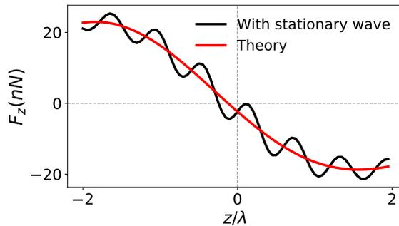
FIG. 8. Axial force exerted on a polystyrene sphere of radius  $r = 0.1\lambda$  with theoretical BSC  $A_n^m$  (black) and theoretical BSC with a counter propagating wave with 0.5% amplitude (red). (color online)
