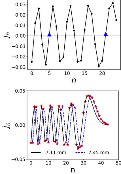
FIG. 3. (Top) Amplitude of the spherical Bessel  $j_n(kr)$  function for a radius  $r = 7\text{mm}(5.6\lambda)$  (the blue triangles show the values close to zero) and (Bottom) for two different radii  $r_1 = 7.11\text{mm}(5.7\lambda)$  and  $r_2 = 7.45(6\lambda)$  (the red points show the maximum values between  $|j_n(kr_1)|$  and  $|j_n(kr_2)|$  for each order  $n$ ). The frequency is  $f_0 = 1.2\text{MHz}$ . (color online)
