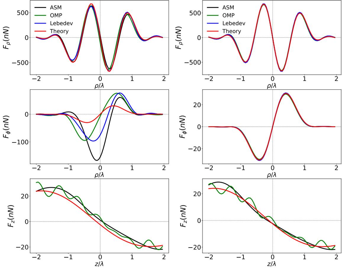
FIG. 12. Experimental radial  $F_\rho$ , azimuthal  $F_\phi$ , axial  $F_z$  forces exerted on an polystyrene sphere of radius  $r = 0.1\lambda$  in a focused vortex beam with charge  $m' = 1$ , calculated by the total coefficients (Left), and only by the BSC in column  $m = 1$  (Right). (color online)
